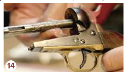
14 Centaur conversion: application of Vaseline to the arbor before shooting blackpowder cartridges.
