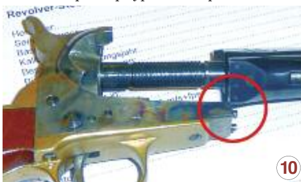
10 Checking out the length of the arbors in Italian Colts ... this one is too short!
