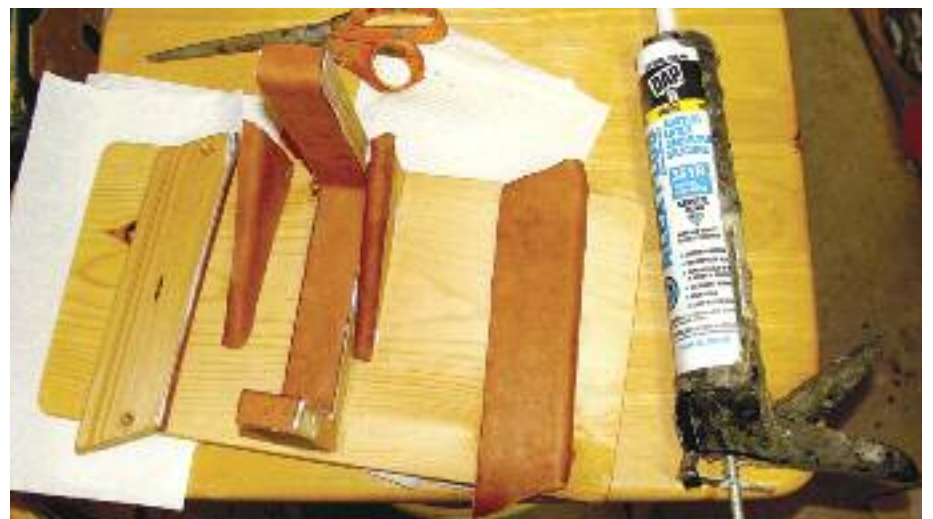
Applying the deerskin to the inside of the stand using DAP ACRYLIC SILICONE CAULK. The leather helps to keep from marring the gun and cushions the piece in the stand.
