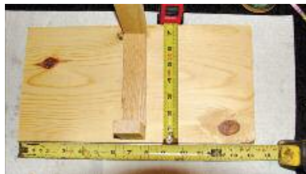
Base measurements. The corners are rounded off to around a 1/2-inch radius. If you bring out the grain, sand, stain, apply one coat of finish, sand, and apply second coat of finish, it'll look great and last quite a spell.
