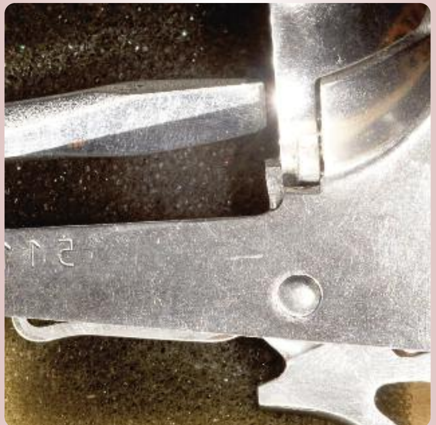
Depressing The Projecting Arm Of The Gate Detent Spring With A Screwdriver Showing The Curved End That Will Be Pushed Back Into The Frame.
