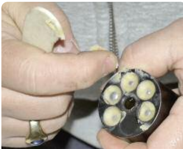
Chamber sealing with HP .357 provides additional lubing
