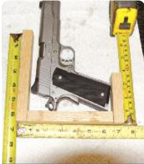
Measurements for the stand. The bottom piece fits between the two uprights and should be cut a little longer than the height of the pistol plus deerskin padding on each side, if so desired.
