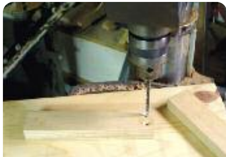
Drilling and counter sinking holes for the uprights. The stand is held together with caulk and wood deck screws.
