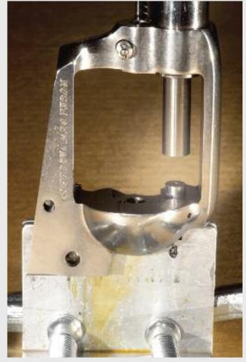
Figure 12. Driving The Recoil Plate Assembly With Firing Pin Above The Corresponding Recess In The Fabricated Base
