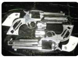
The process to prepare the gun for the new finish is to completely disassemble the firearm. After disassembly, the individual parts are degreased. Preparation for the application involves grit blasting the surfaces of each part to a satin like finish. Then plugging the bore and chambers.
