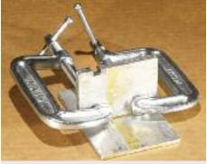
Figure 11. Fabricated Base For Recoil Plate Installation
