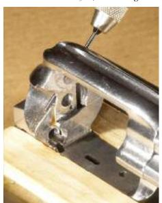
Figure 10. Follow-Through Drilling Of Existing Recoil Plate Cross Pin Hole To Remove Residue and Cuttings Showing Drill Exposed In The Recoil Plate Recess
