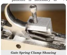
Relationship Of Allen Head Screw To Loading Gate Detent Spring
