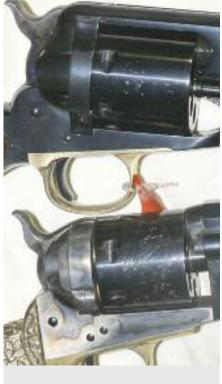
Hammer resting on an empty chamber? Difficult to see on Uberti Remington (top), but no issue with Uberti Colt Navy-conversion (bottom)
