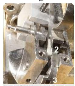
Partial Removal Of Trigger/ Cylinder Latch Pivot Pin Showing: (1) The Recess In The Pin That Is Held By The Gate Detent Spring, (2) Trigger And Trigger Recess Into Which Trigger Spring Fits, And (3) Hammer Recess For Strut
