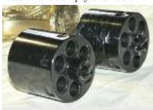
Recesses for the cartridge rims of Uberti Remington conversion (left) and "flat" breech side of chamber of Uberti Colt conversion (right)
