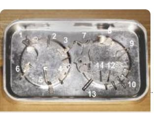
Ruger Small Parts: # 1 - Trigger # 2 - Trigger / Cylinder Latch Pivot Pin #3 - Cylinder Latch # 4 - Recoil Plate, Recoil Plate Cross Pin, Firing Pin, Firing Pin Rebound Spring # 5 - Transfer Bar # 6 - Pawl #7-Hammer with Hammer Plunger and Hammer Plunger Pin #8 - Loading Gate #9 - Loading Gate Detent Spring #10 - 5 x Grip Frame Screws #11 - Cylinder Latch Spring and Cylinder Latch Spring Plunger #12 - Pawl Spring and Pawl Plunger #13 - Hammer Pivot Pin
