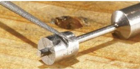
Figure 8. Filing the Recoil Plate Channel
