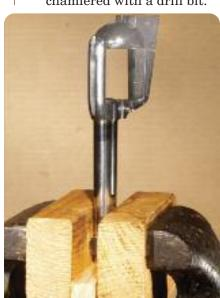
Wood Block Arrangement In Vise For Driving Out Recoil Plate
