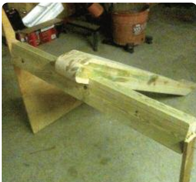
Axle and tongue frame. First step in building the carriage.
