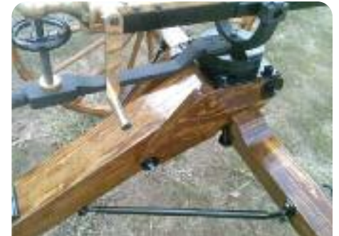
The crank is in the foreground and the elevation screw in the back. After the adjustments are made, the gun can be moved a little when it is fired.
