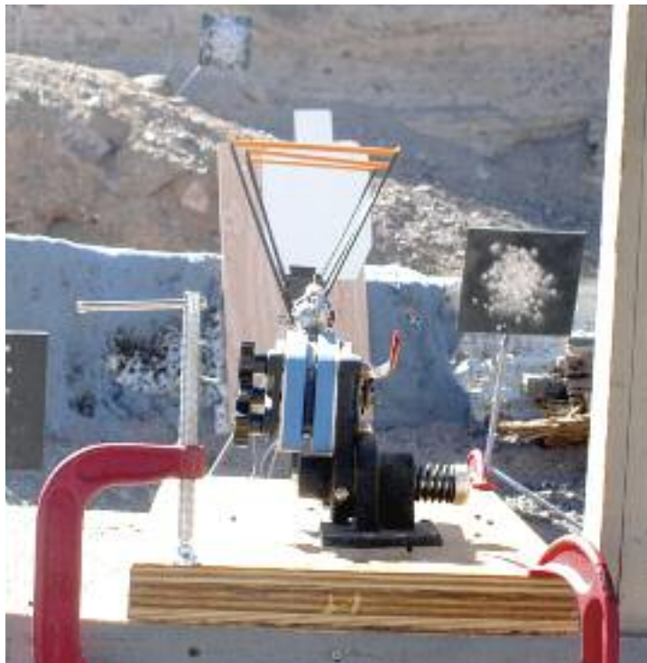
The Ransom Rest is clamped to a shelf at Cowtown in Phoenix. In front of it are the three screens of the Oehler 35P Printing Chronograph, then a target.
