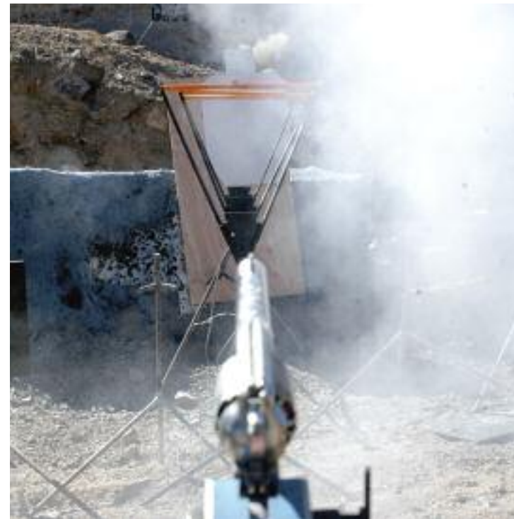
Firing the Ruger Old Army in the Ransom Rest. The rest allows the gun to recoil and has to be pushed back to its stop for the next shot.
