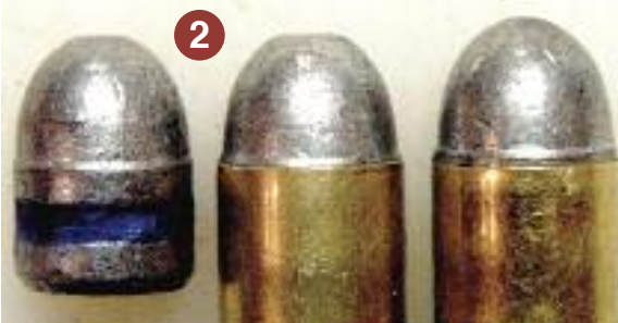
Photo 2—Left to right: A 230 gr. LRN bullet; a round with the bullet correctly seated and crimped; a round with the bullet seated too long and the brass crimped into the lead.
