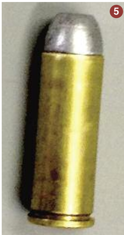
Photo 5— .45 Colt with 200 gr. LRNFP bullet correctly loaded. Note roll crimp into the crimp groove.
