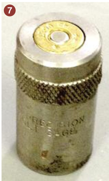
Photo 7— .45 Colt Chamber checker/case gauge with a round that passed inspection.
