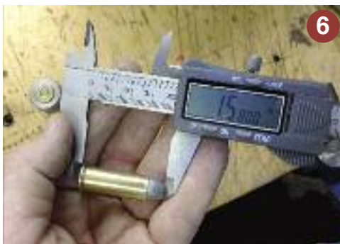
Photo 6— I've locked the caliper at 1.58". Any round that passes through will fit in my Cimarron Uberti '73 made in the 1990s.
