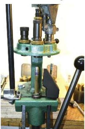
Round is at station 4, ready for bullet seating. When the bullet is seated at station 4, the round is complete—unless ...
