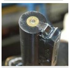
Chamber checking a completed round in a barrel that has been removed from a H & R.
