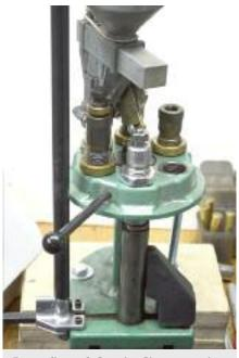
I use five of the six die mounting holes in the RCBS Turret Press-(1) Lee De-capping/resizing die, (2) RCBS Cowboy expander die with the large expander plug, (3) Dillon Powder measure die, (4) RCBS Cowboy seating/crimp die, (5) RCBS Cowboy de-capping/ resizing die with de-capping mechanism removed to resize completed round.
