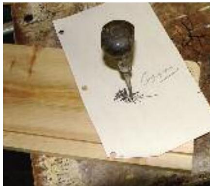
Thin cardboard used for locating the cart hinge point. The top back of the tray had to be rounded over to allow the rack to clear when folding down.
