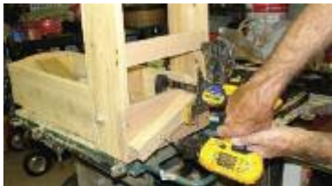
Locating/drilling holes in oak lower back plate of gun rack.
