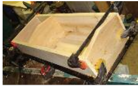
Tray glue up. The tray is used for an ammo box, tools, etc.
