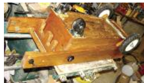
Underside of cart. The rear axle had to be moved all the way to the back of the tray o keep the cart stable.
