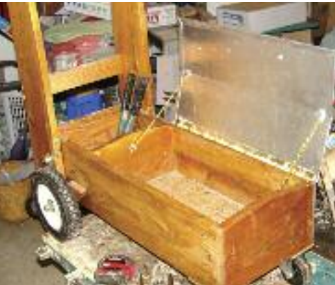
The metal cover is bent to fit the slope of the tray top. A piano hinge works well on the cover. Small screws hold it to the wood and pop rivets to the metal. A small metal angle was used for a ridge pole.
