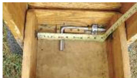
View of parking break in bottom back of tray. The long gun butt space in back of tray is lined with deerskin. There are small woodblocks screwed in place that hold parking brake rod in park or moving position. I used 3/8" DIA. steel rod, but 5/16" DIA. should suffice.
