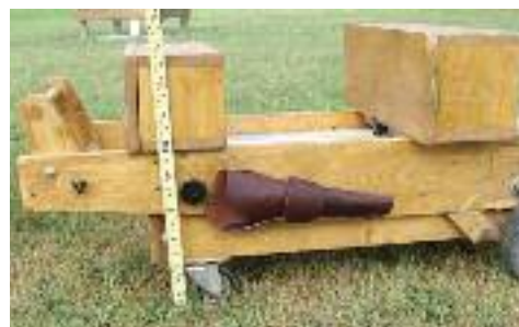
Side view of folded cart. Notice the position of the thumb screw. Holsters are placed on each side of cart.
