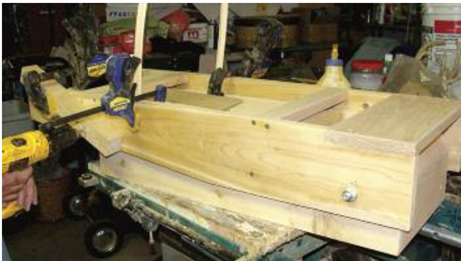
Locating/drilling holes for the thumb screws in lowered position. To help keep the holes perpendicular to the surface, a piece of wood was drilled in a drill press and then clamped to the board to be drilled.
