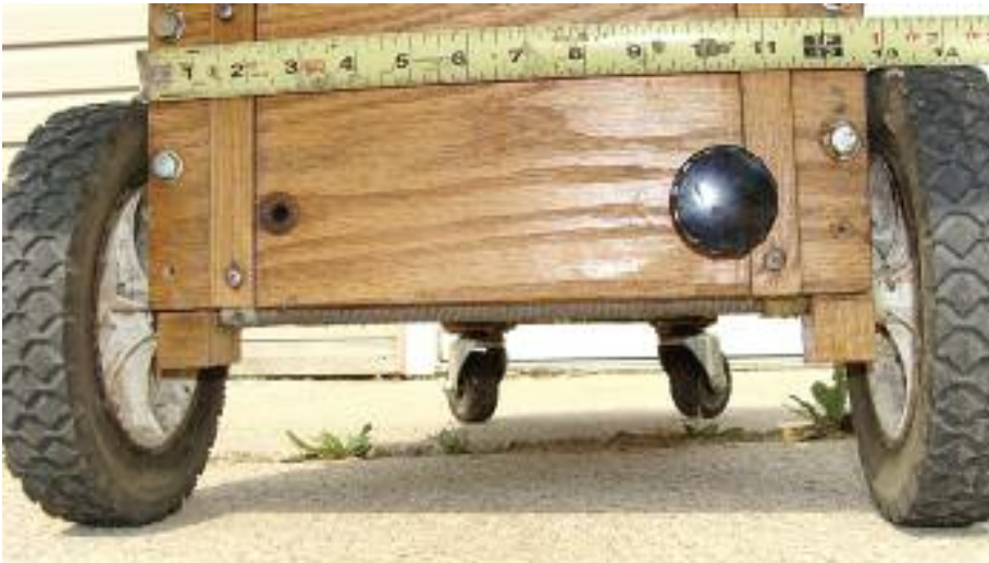
Back bottom of upright cart. Notice the 1/2" threaded rod axle is at the very rear of the tray.
