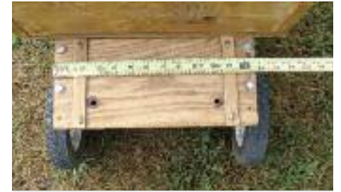
Oak is used on the bottom/back of the gun rack for extra strength. Holes are placed in it for the thumbscrews.
