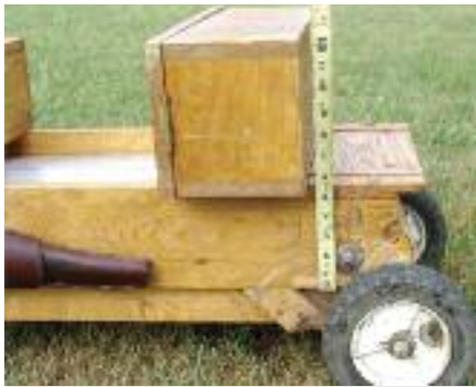
Cart in down position. Notice the bottom of the gun rack (at right) is rounded to allow it to miss the rear axle when folding.
