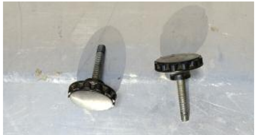
5/16" x 2" long thumbscrews used to hold the cart upright and to hold it folded down for transportation.
