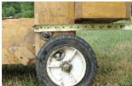
Cart in upright position. Notice the bolt for the pivot point and the rod through wheel setting the parking break.
