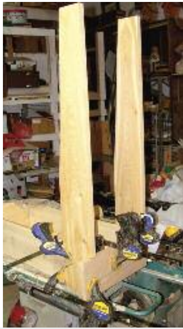
The oak board is placed at the lower part of the gun rack.
