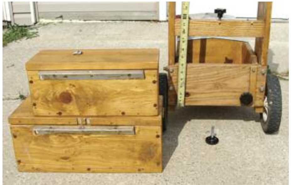
Horizontal measurement view of bottom/back of cart. The boxes sitting at left can be taken off by removing one wing nut. There is a 1" aluminum angle secured to the back of the boxes. One 5/16" stud in the center and two equally placed 3/16" studs connect each box to the cart.
