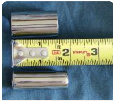
Plated coupling at top and tip at bottom. The coupling is around 1-5/8" long (Made from a 3/4" copper pipe solder coupling) and the tip is around 2" long (Made from 1/2" copper pipe).
