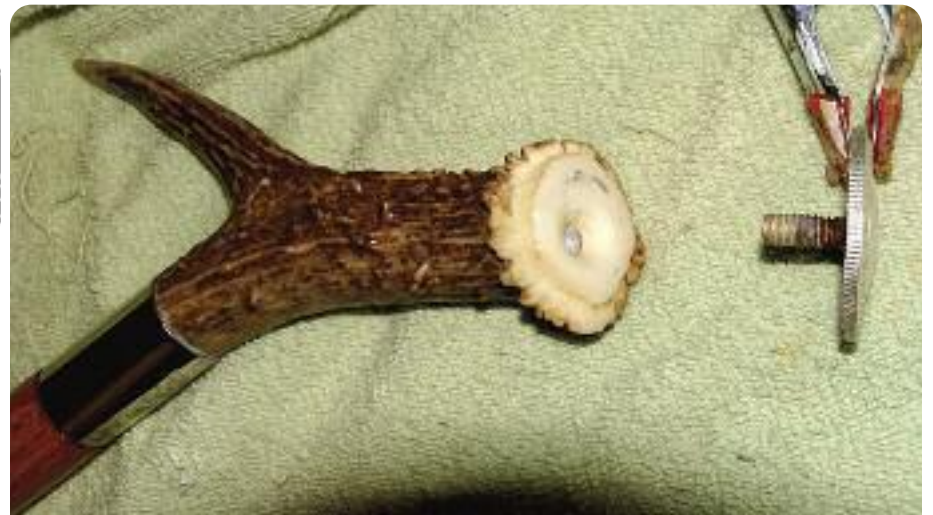
The coin was made concave using a ball peen hammer and appropriate sized holes made in a piece of wood that holds the coin in place and at the same time allows the coin to be depressed to the form of the antler drop. The silver coin has a 1/4"-20 TPI X 5/8" long flat head brass machine screw soldered on center to its concave side. The antler drop end is drilled, tapped, and counter sunk on center at the correct angle to accept the coin screw. Some type of marking was used to show the high spots on antler; then it was filed down to assure correct fit. If coin is not wanted, the antler drop end can be filed, sanded, and polished smoothed.
