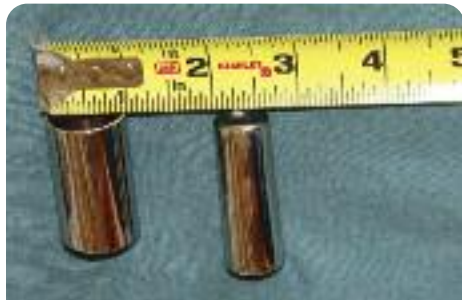
View showing the outside diameter of the coupling and tip bottom. The coupling is around 1" outside diameter. The tip is around 5/8" outside diameter at its bottom where the hole is drilled in it and around 3/4" outside diameter on the end that slips onto the wood shaft bottom.
