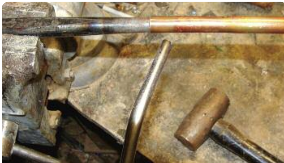
The tip was made out of 1/2" copper pipe (5/8" outside diameter). A long tapered drift was firmly secured in a vise and a short piece of the copper pipe was slipped over it, heated, and tapped onto drift until the outside diameter was around 3/4" for the top end. Then the pipe was cut to around 2" long. A brass patch was soldered into the inside bottom of the tip and a hole was drilled in it to fit the size of screw that was used to hold the tip onto the shaft. An appropriate sized washer could also be soldered in. The coupling is around 1-5/8" long and was made from a 3/4" copper pipe solder coupling that is around 1" outside diameter. Next, they were plated.
