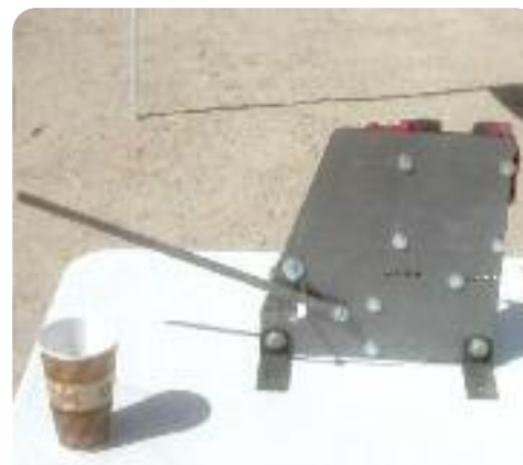
Front and back views of the kicker. The “long arm” on the front is the trigger and the “flipper” is mounted on the back.
