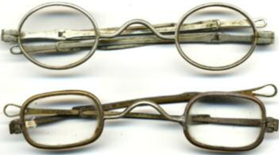
Examples of inexpensive spectacles made of brass and German silver. Top: Oval German silver spectacles with loop slide temples. The joints are the most common type, using a screw to hold the joint halves together, and a separate pin for the temple pivot. Bottom: Oblong brass spectacles, German silver bridge and loop slide temples. This is the other common joint of the period. The single screw holds together the joint halves and also serves as the temple pivot.
