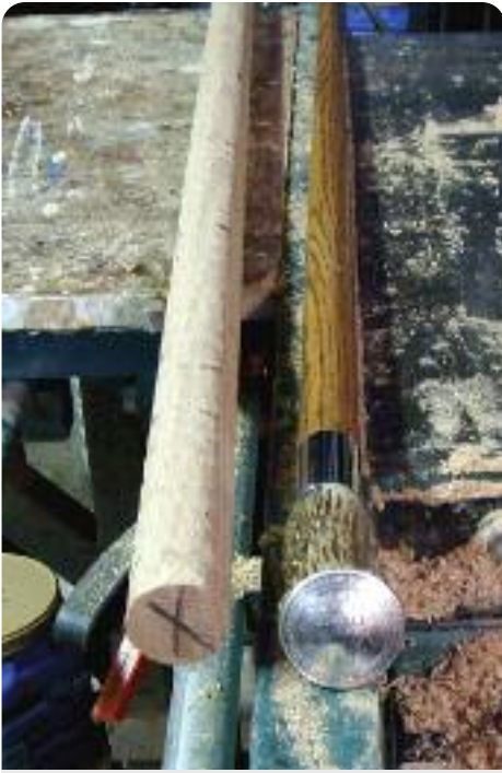
Roughed in cane shaft along side finished one. I aim at roughing in the shaft diameter size to around 1/16" over size and then sand to size (including bringing out the grain).
