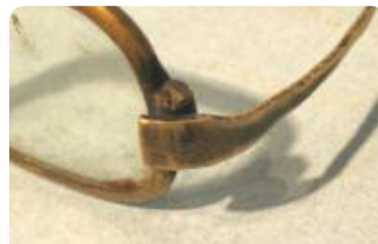
Close-up of the single pin joint found on inexpensive spectacles.
