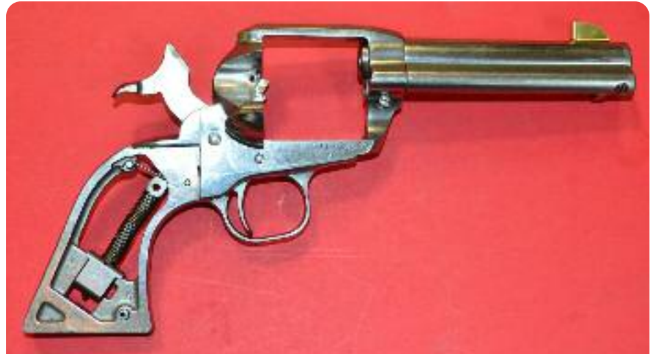
Ruger Vaquero frame with Shotgun Boogie’s “Game Changer” Short Stroke kit. Gun is at full cock.
