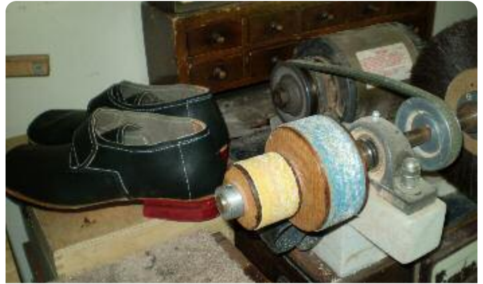
My shoemakers rollers and sanders. If inclined, hook a rig up to a 1500 or 1700 rpm forced air furnace motor.
