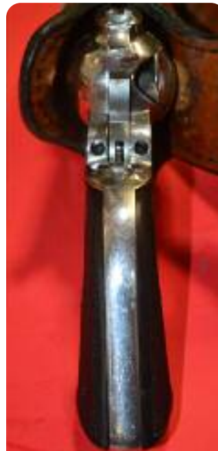
End view of stock Ruger grips. Note they flare toward the bottom.
