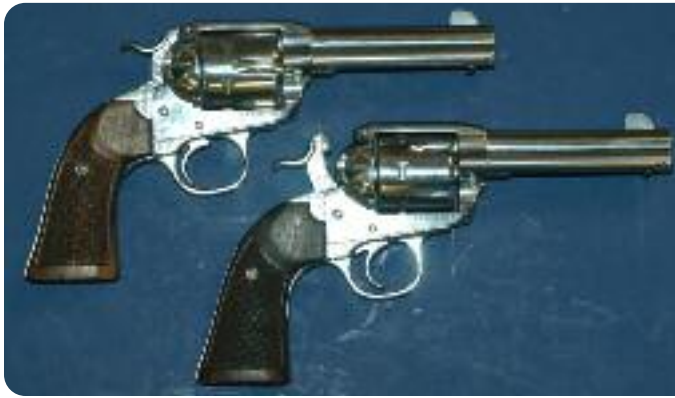
Vaquero by Jimmy Spurs of Cowboy Gunworks converted to Bisley grip frame and hammer with light, smooth action job and light trigger, transfer bar removed and half-cock notch. Bottom gun is on half-cock.
