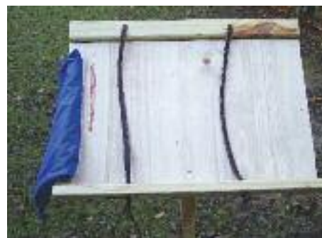
Modified version. A piece or two of thin plywood covers the frame
