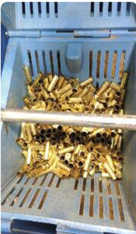
Tumble it in your brass tumbler for 3-4 hours, and it comes out looking as good as tumbled smokeless brass.
