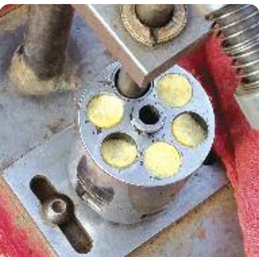
Photo 5 – Then the cylinder is moved to the Cylinder Loader and Wonder Wads are inserted and seated. The rammer is inserted into the “empty” chamber so you load the correct ones. If you’re using American Pioneer Powder or Hodgdon Triple Seven, Wonder Wads are not used, saving about 30-50¢ per cylinder and one step in loading.
