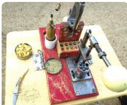
Photo 7 – Then the balls are placed on top of the chambers and the rammer is centered on the first ball.
