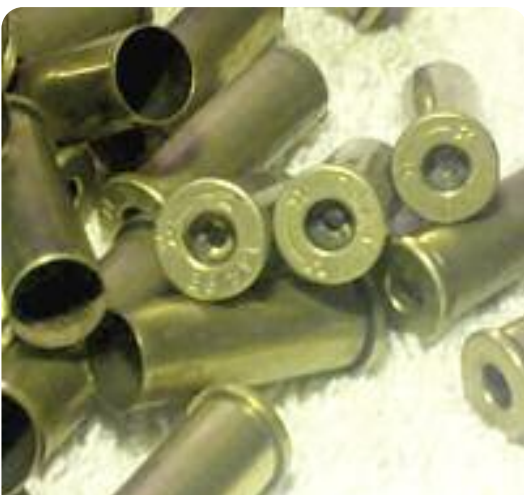
Note the carbon in primer pockets and how dark they are on the inside. We are about to fix this problem.
