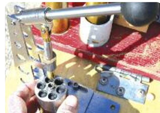
Photo 9 – After loading a cylinder, the chambers have thin lead rings on the tops from compressing oversized balls into the chambers. These rings are wiped off before the cylinder is reinstalled in the frame.
