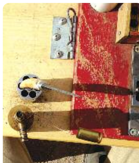
Photo 4 – The Screwknife "chases" the chamber to be loaded until all five are loaded. This helps avoid double charges or no charges.
