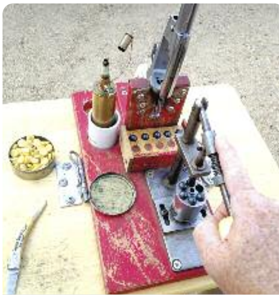
Photo 8 – Then the balls are seated.
