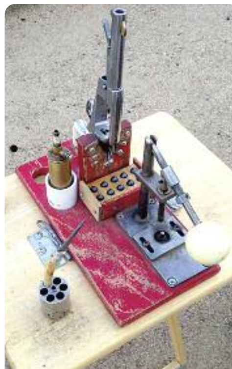
Photo 3 – The loading sequence. The Screwknife is inserted into the "empty" chamber, and powder is inserted into the chamber on its left. Then the Screwknife is moved to that chamber, which verifies that there is actually the correct amount of powder in the chamber, and the next chamber gets powder.
