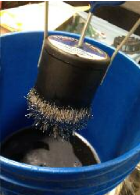
The Frankford Arsenal Media Transfer Magnet picks up media from the water used to clean the last batch of brass.
