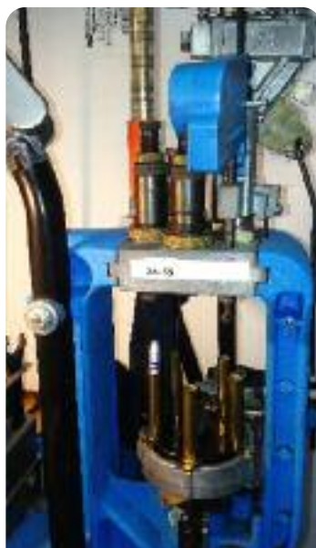
Dillon XL650 set up for .38-55 Winchester.
