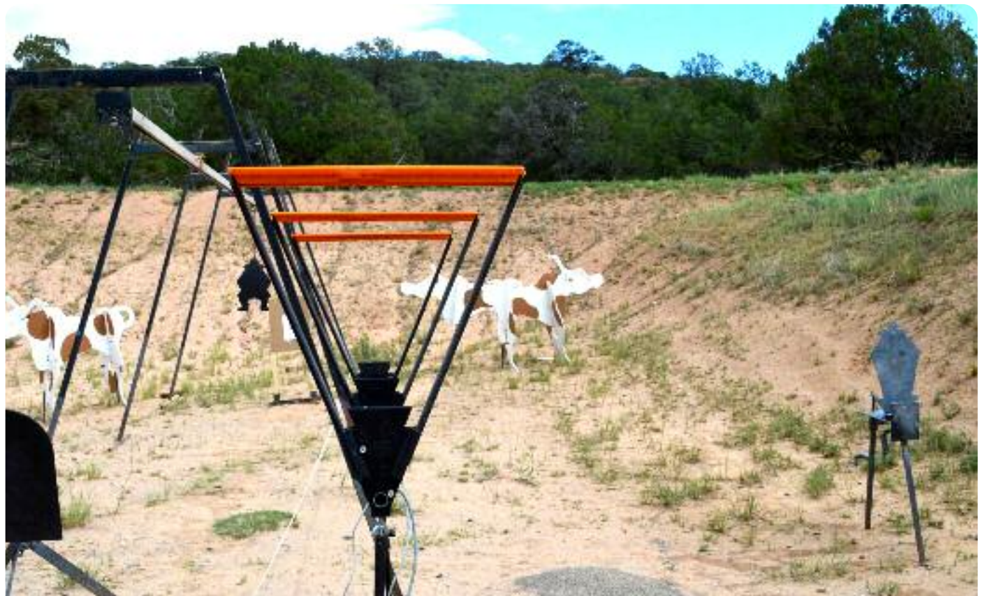
The view through the three screens (proof screen in the middle) of the Oehler 35P Printing chronograph.
