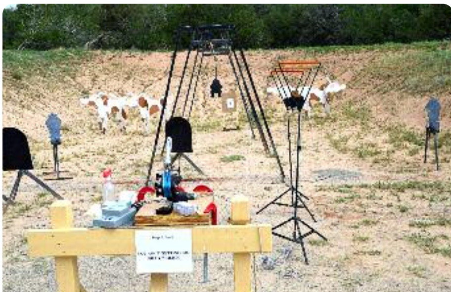
Looks complicated, doesn't it? It's not. The fence table was bolted down and immovable, making it a perfect mount for the Ransom Rest. The targets were set for a match the next day, so I worked around them. Unfortunately that table is too close to the ground for the tripods for the Oehler 35P Printing Chronograph's screens, so it was set up nearby, and one Ruger Vaquero was shot groups from the Ransom Rest, and the other was shot for chronographing. No plywood cattle were harmed during the making of this test session.
