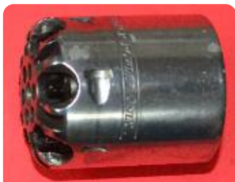
BEFORE: ROA Cylinder crusted with cap residue.
