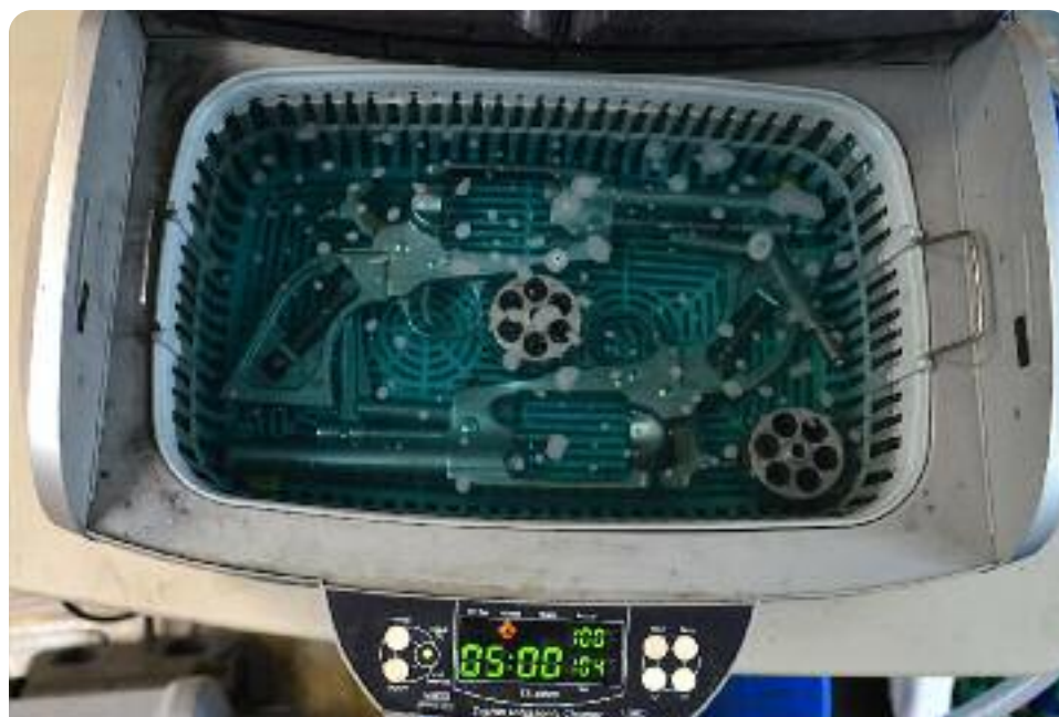
DURING: 2 ROAs and cylinders in Lyman 6000 Turbo Sonic cleaner with Lyman Turbo Sonic steel parts cleaner and water.
