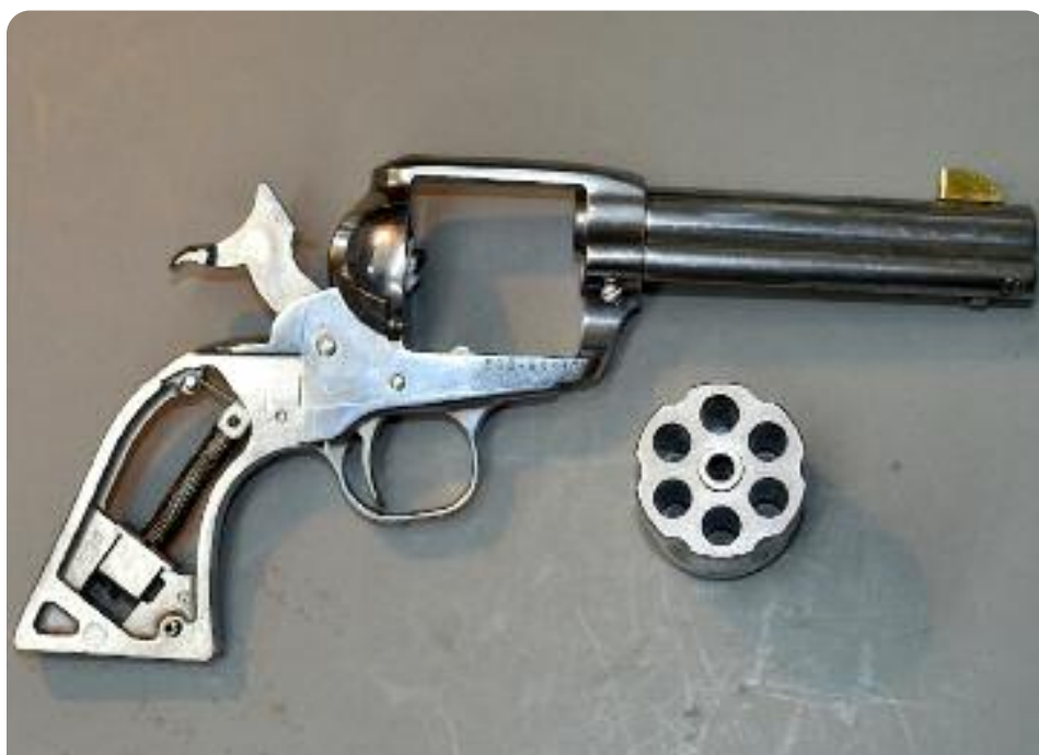
Stainless Ruger New Vaquero very clean after 15-minute sonic soak, BUT there were internal rust problems the next day. Sonic cleaning removes all oil, and flash rust can result. OIL ENTIRE FIREARM IMMEDIATELY on removing from bath.
