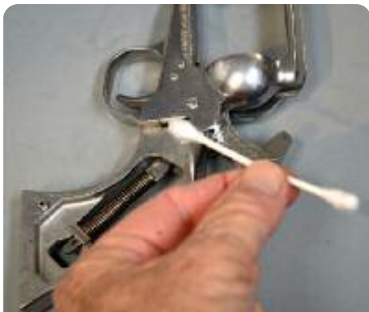
AFTER: Q-tip picks up nothing when run through hammer slot.
