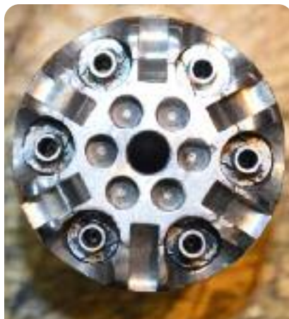
AFTER: Cylinder and nipples much cleaner. But when nipples rotated 180°, crud was still found on inside, requiring light brushing to remove.
