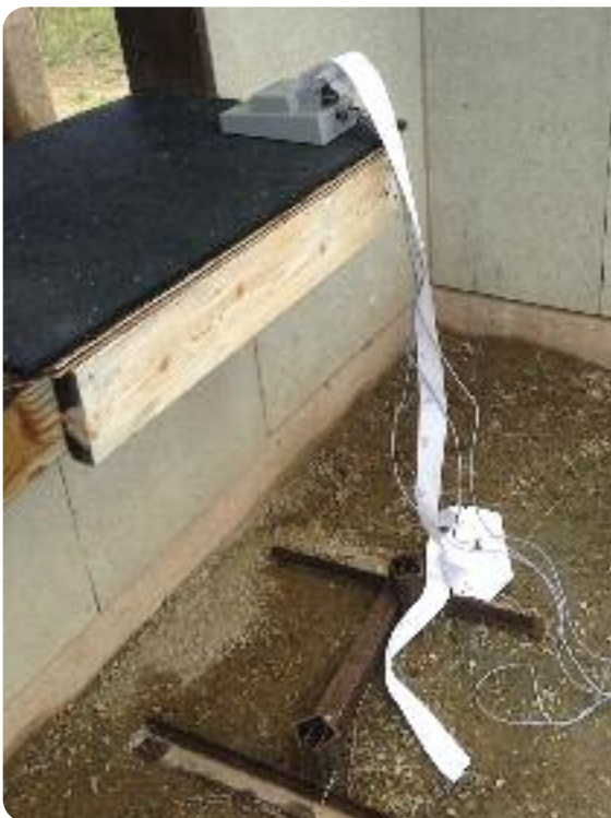
Chronograph testing used an Oehler 35P Printing Chronograph. The tape tells the tale.
