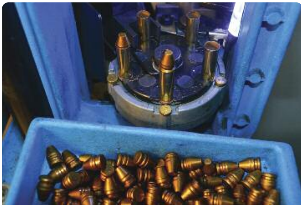
Loading 105-grain bullets on Dillon XL650.
