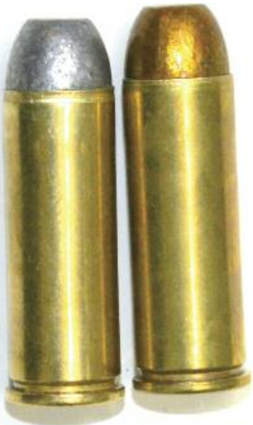
Comparison of 200-grain LRNFP and 200-grain coated RNFP in loaded ammunition.
