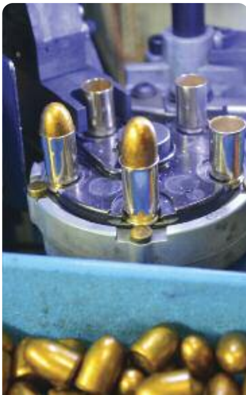
Loading coated .45 ACP 230-grain RN bullets.
