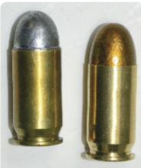
Coated 230-grain RN vs. lead 230-grain RN in loaded ammunition.
