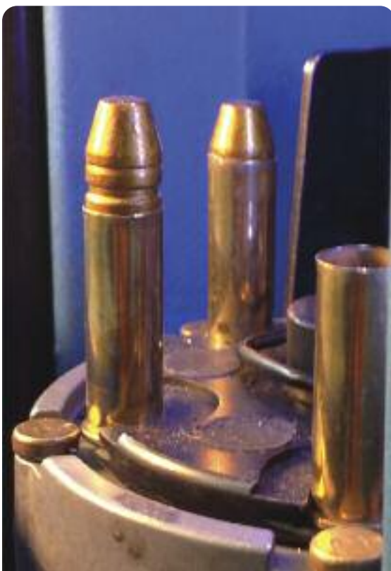
Loading 125-grain FP bullets. Note the case mouth has been belled just enough for the round to sit inside the mouth.
