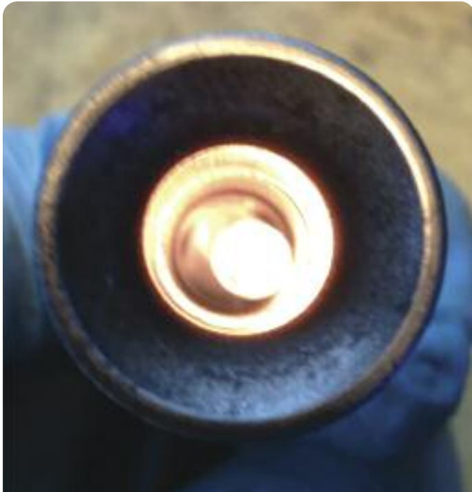
Crimping die after loading 500 coated bullets.
