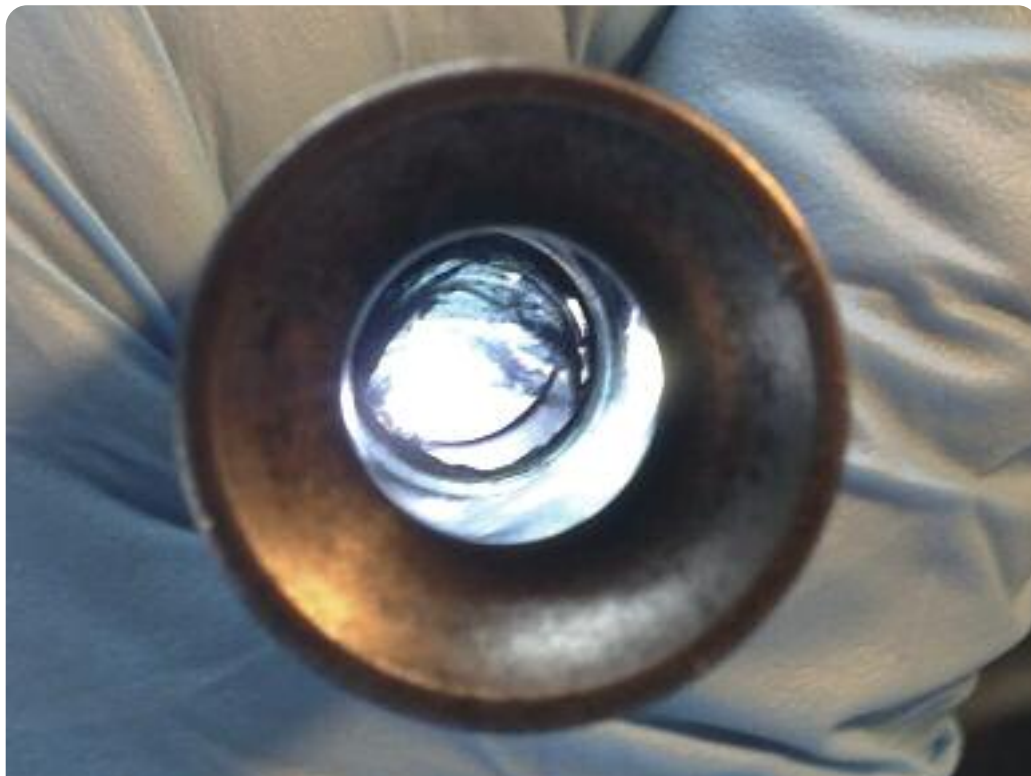
Crimping die after loading 300 lead bullets—needs to be cleaned to remove bullet lube.
