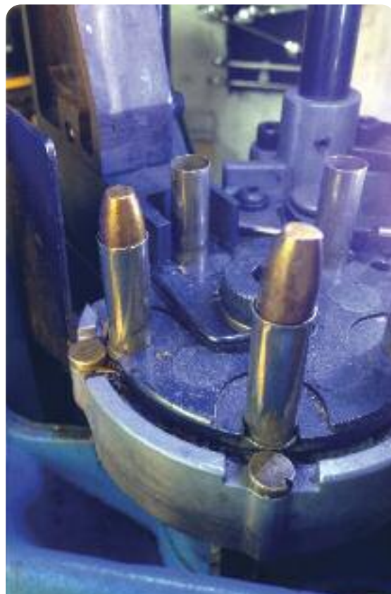
147-grain FP bullets have no crimp groove, adding to their versatility. OAL can be adjusted to suit your rifle.
