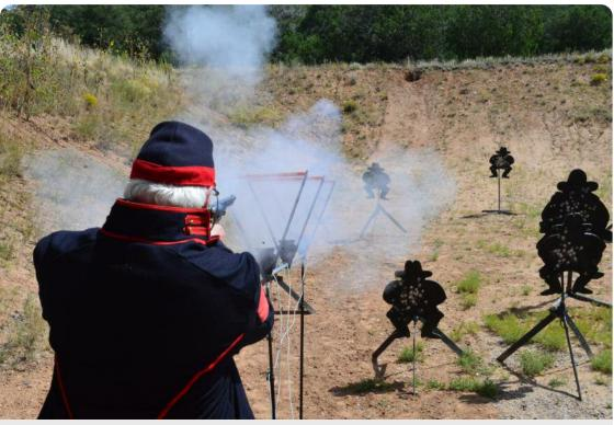
1847 Walker, .44 cal., 60 grains FFFg. This is a chain fire. The next chamber fired just after the one under the hammer, ba-bang. No damage.
