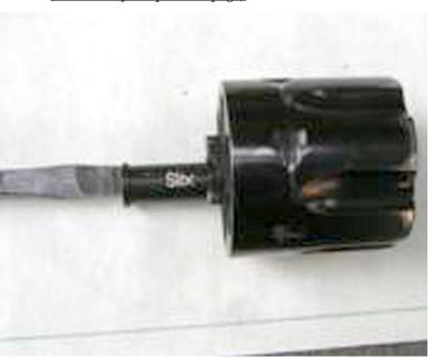
ber. To remove the collected *ejecta* from any pistol cylinder chamber, merely place the SliX-Scraper into the chamber and, using a thin slotted screw-driver turn it to the *LEFT*! In either case you can easily feel when the chamber is clear. Please see the
