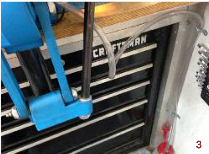
The tube from the Spent Primer Chute needs some “slack” when the handle is up. I substituted 1/2" PVC tubing from Home Depot because I needed more than three feet.
