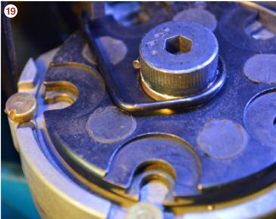
Addition of a bearing atop the shell plate.
