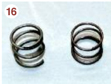
13 Improved case feed ram cam follower with bearing on the left, standard on the right.
