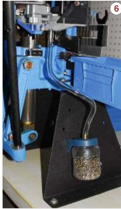
If you use a Dillon Strong Mount, dillonupgrades.com makes a spent primer chute that works neatly with it.
