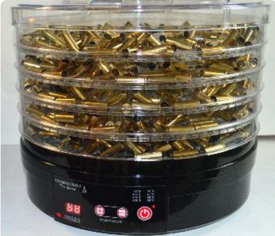
CED Brass dryer with all five trays loaded with 750 rounds of .38 Special brass. It's at 68°C. After 30 minutes brass was dry and not too hot to pick up, if in doubt, let it cool before transferring.
