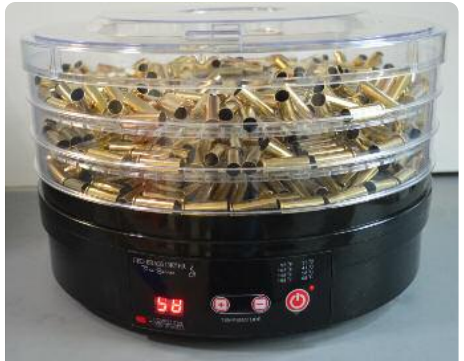
CED Brass dryer with four of five trays loaded with brass. Temp gauge shows 58°C.
