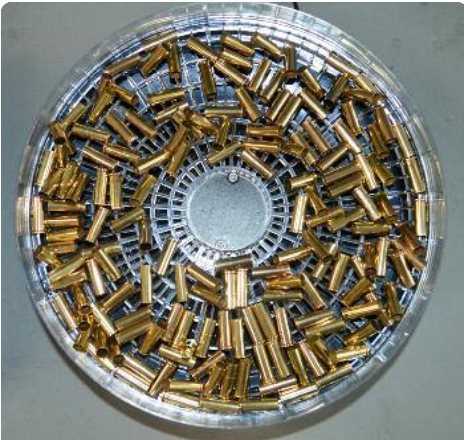
One of five brass dryer trays loaded with one layer of .38 Special brass (165 rounds).
