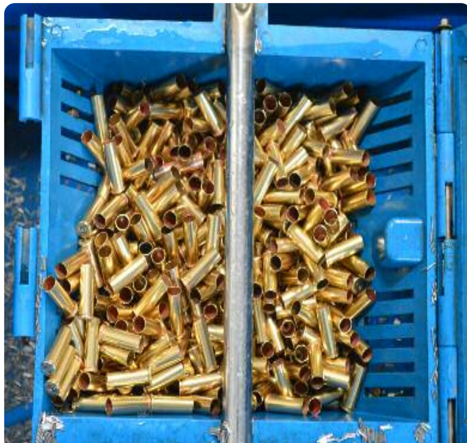
Brass cleaned in stainless media in a rotary tumbler then "spun dry" in a media separator.
