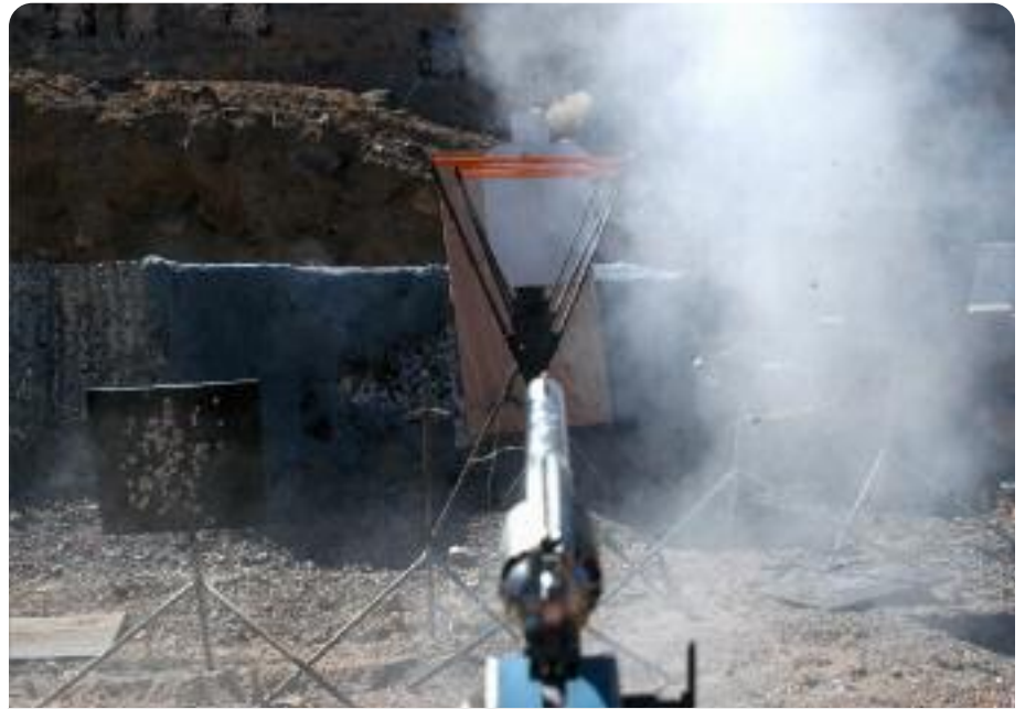
We’ve done considerable range testing of guns, ammunition, powder, and bullets. In January 2013 we tested several black powders and substitutes using a Ransom Rest and Oehler Chronograph.
