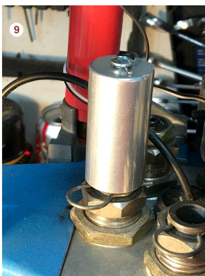
the other half of Unique Tek's Loaded Round Counter. This unit is placed on the crimping die. It has a magnet in the bottom to hold it in place. When the round pushes the rod up...
