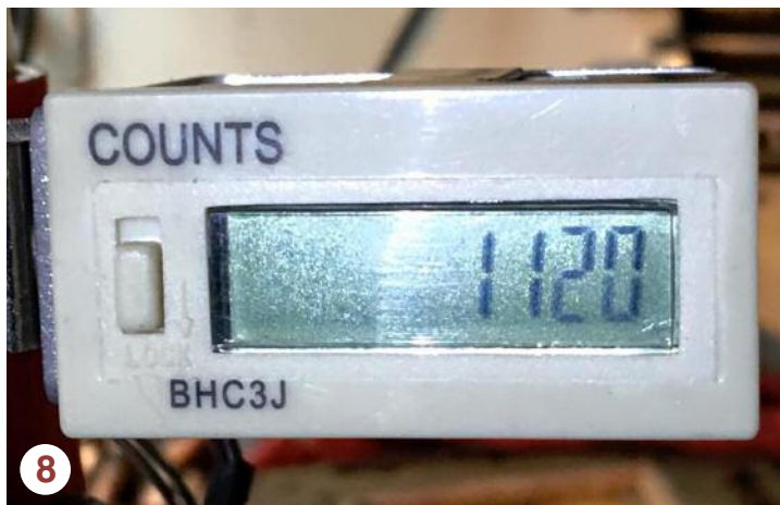
Unique Tek's Loaded Round Counter. Mount the counter on the primer tube, and...
