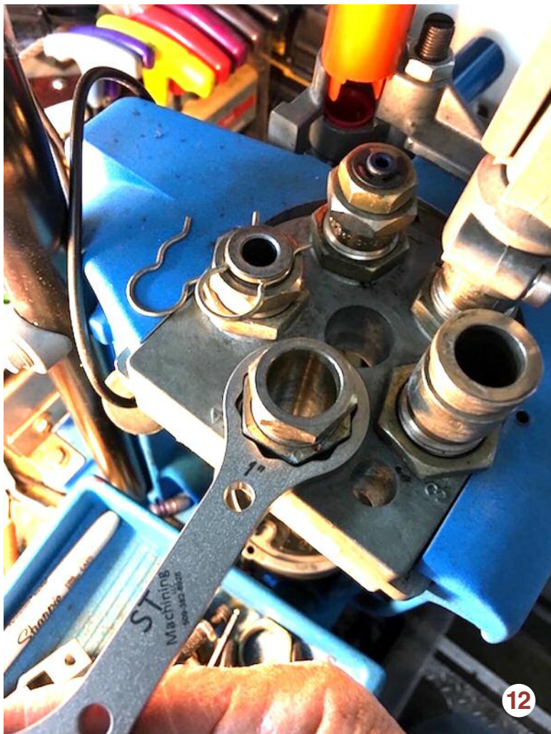
Wrench fits closely-spaced die lock rings, One of these wrenches is a must have.
