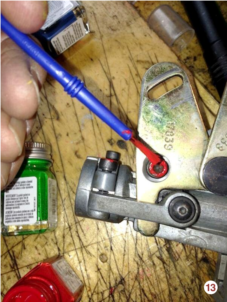
A really cheap trick, requiring only a few bottles of Testor's enamel model paint and some brushes. For each wrench check every socket head. Those that fit that wrench, paint them the same color. Then paint the wrench.
