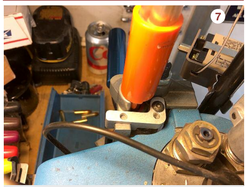
ST Engineering's Case Feed Stop in place. Drop it in place and no more rounds are dropped, but you can work with problems on the shell plate.
