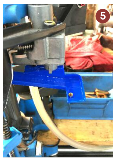
Unique Tek's live primer chute in operation.
