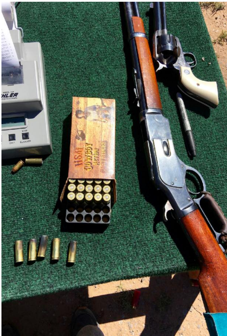
Oehler 35P Printing Chronograph with proof channel and the guns used to test HSM .45 Colt Cowboy Action Ammunition.
