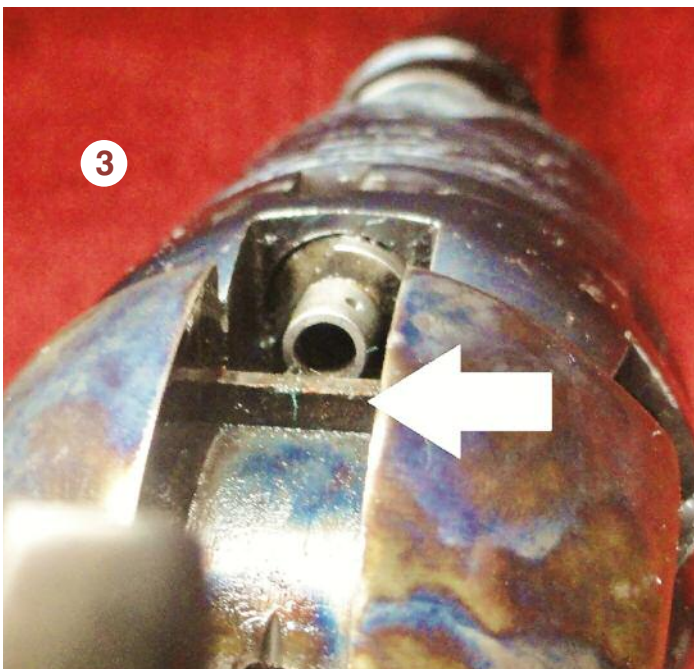
Anti Cap Jam Shelf indicated by arrow.
