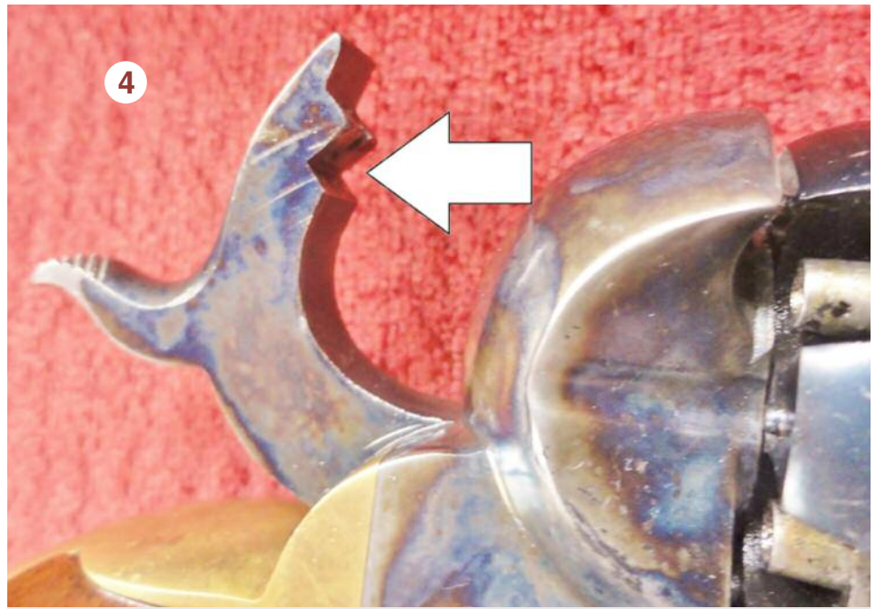
Undercut in hammer to clear the internal shelf.
