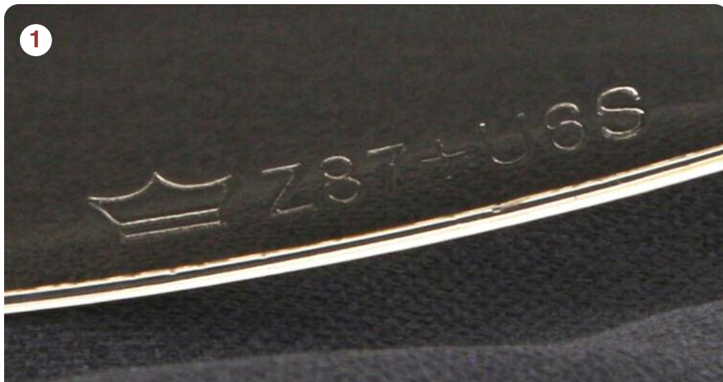
1 Bollé Safety Glasses markings. In this case, the lens is rated: Z87+ indicating maximum Ultraviolet protection (U6) and has a special (S) lens tint.
