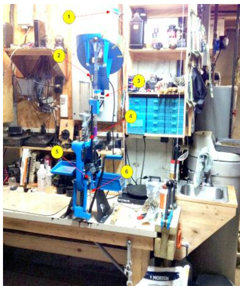
Master setup: 1—Mechanic’s Inspection Mirror; 2—Additional weight for Primer Follower Rod; 3—Round Counter; 4—LED Light; 5—Primer Retrieval; 6—Spent Primer Disposal.
