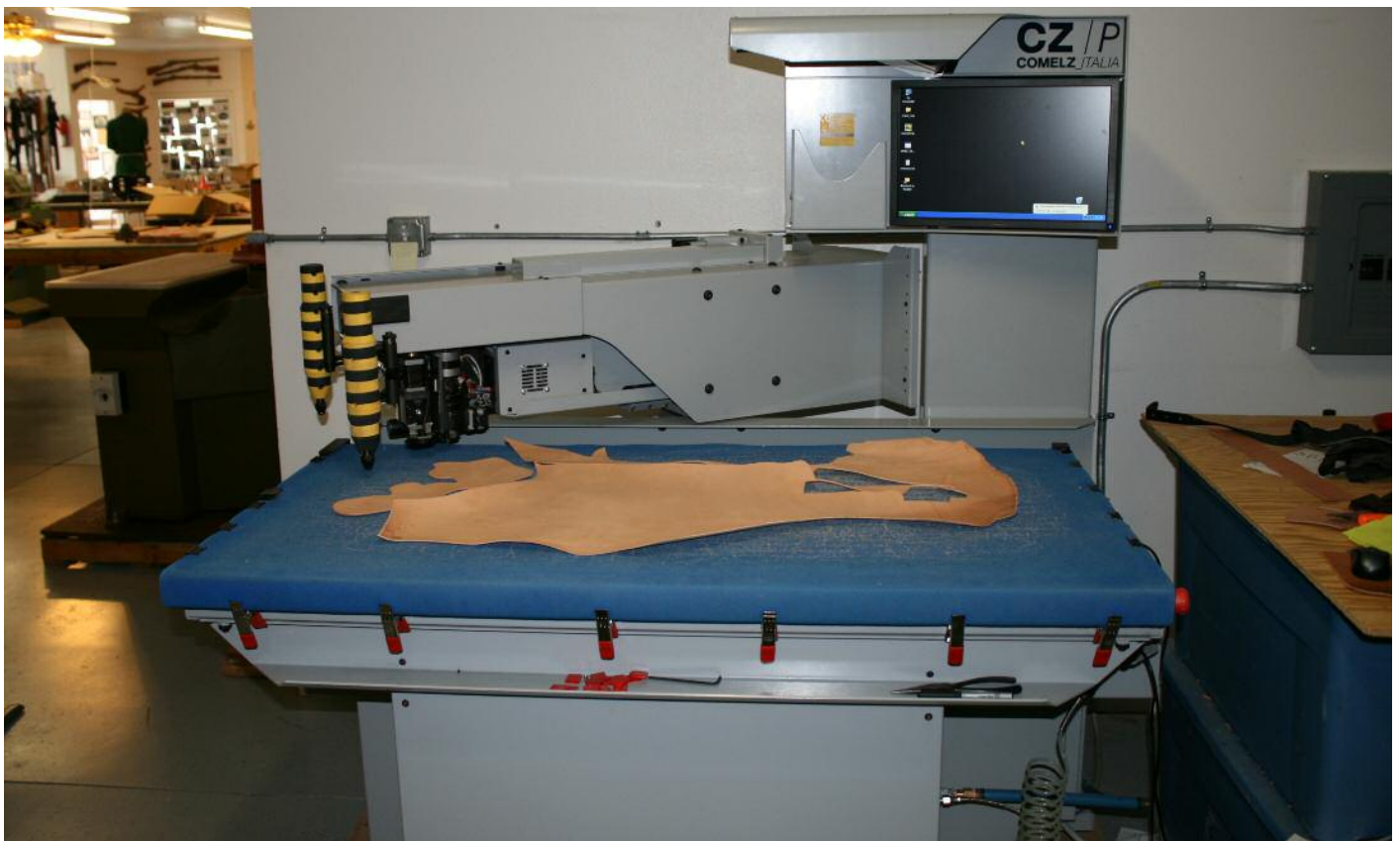
Mernickle Holsters' CNC knife cutting computerized machine that cuts the leather, punches the holes, makes the slots and even draws in stitch lines.
