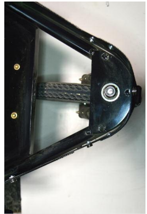
New front end, welded onto frame. The old one was easily removable for storage, but not as sturdy.
