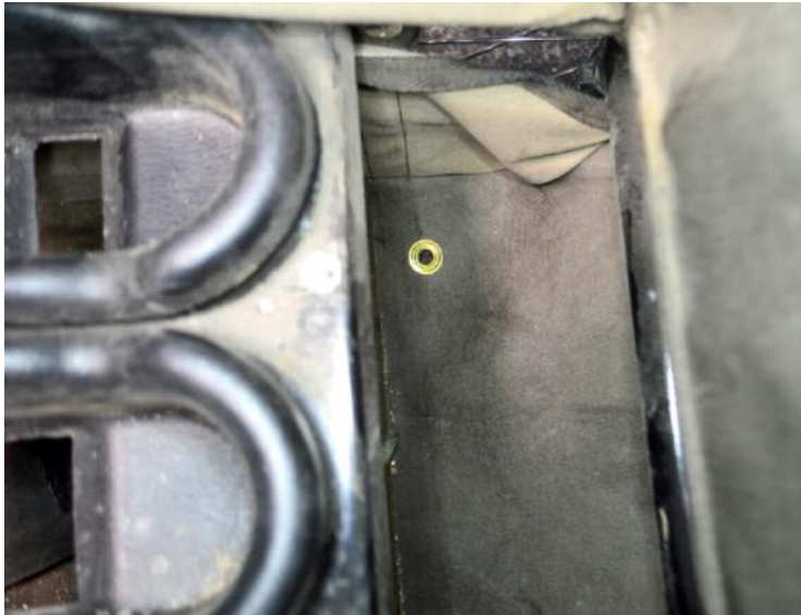
Drain holes in the bottom so the cart won't fill up with water in the rain.
