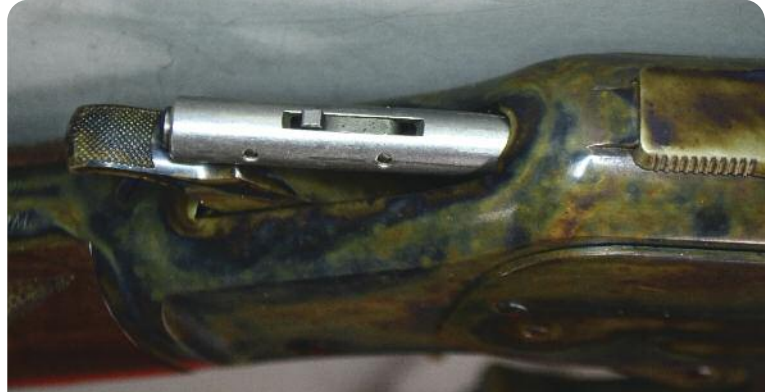
Firing pin safety. Firing pin is blocked until trigger is pulled. Note the beautiful, checkered, case hardened hammer.
