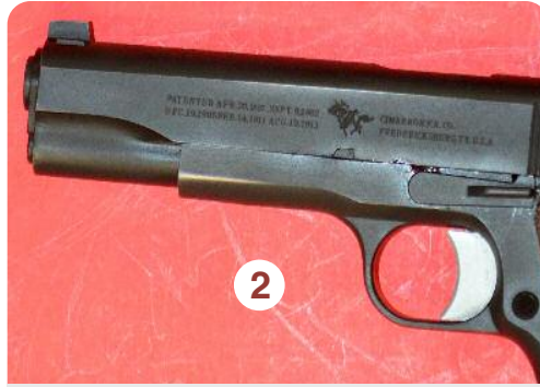
Dovetailed front sight made from a blank.
