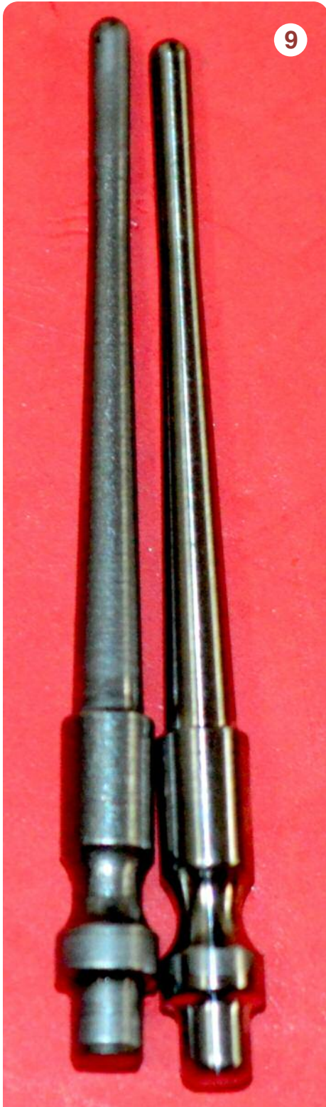
Standard Colt firing pin on left, Wilson "Bullet Proof" stainless steel firing pin on right.
