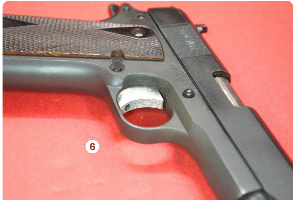
A solid trigger with an over-travel adjustment screw.
