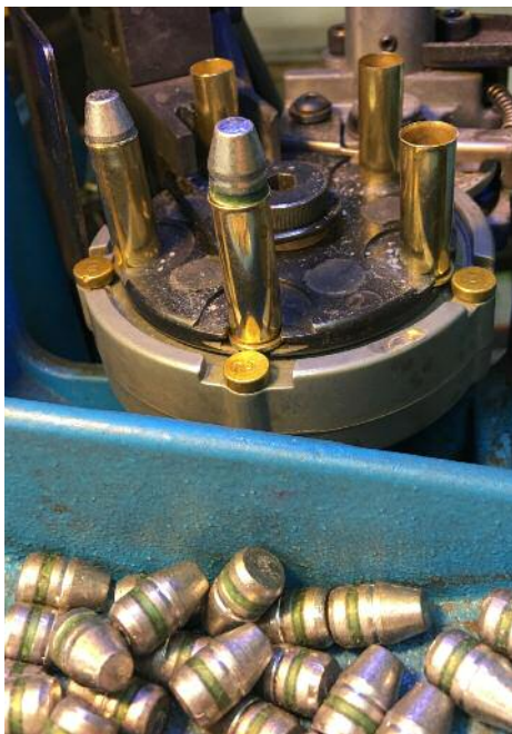
Loading 140-grain .358 diameter LTC in .38 Special. They load just like Laser Cast 125-grain LTC. No adjustments needed.
