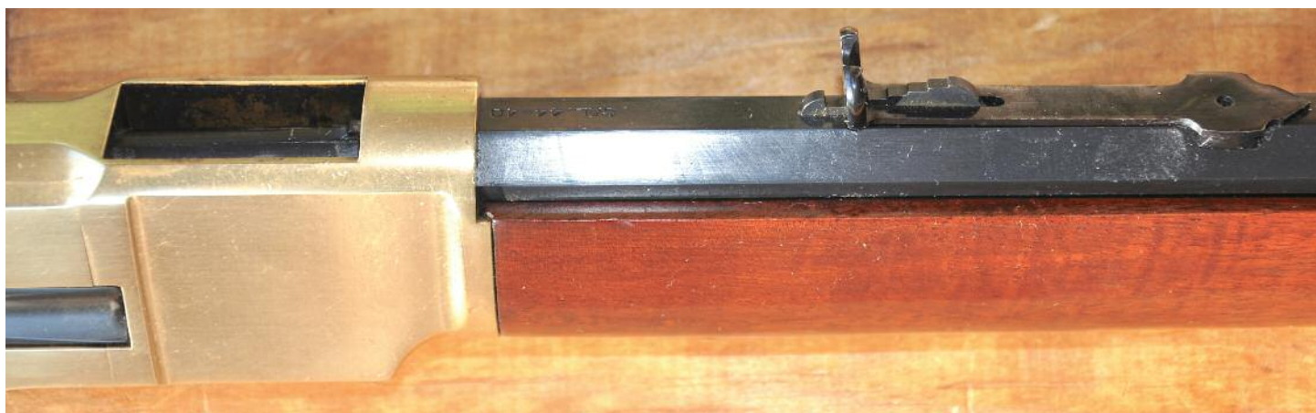
Ejection port on top of receiver and Winchester-style rear sight.
