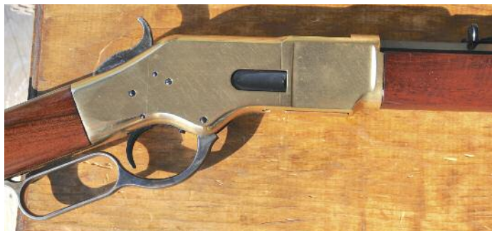
Beautiful 1866 brass receiver with the King's Patent loading gate.
