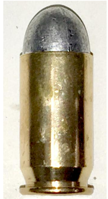
Loaded 230-grain LRN .452 diameter .45 ACP. Taper crimp.
