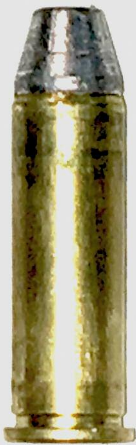
Loaded .38 special 140-grain LTC round. OAL 1.44" with roll crimp in crimping groove.
