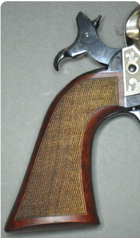
1860 Army grip frame with beautifully fitted checkered wood grips, and lowered and widened hammer.
