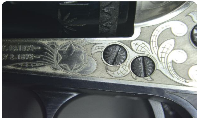
Blued fancy screw-heads are a focal point for detailed engraving.
