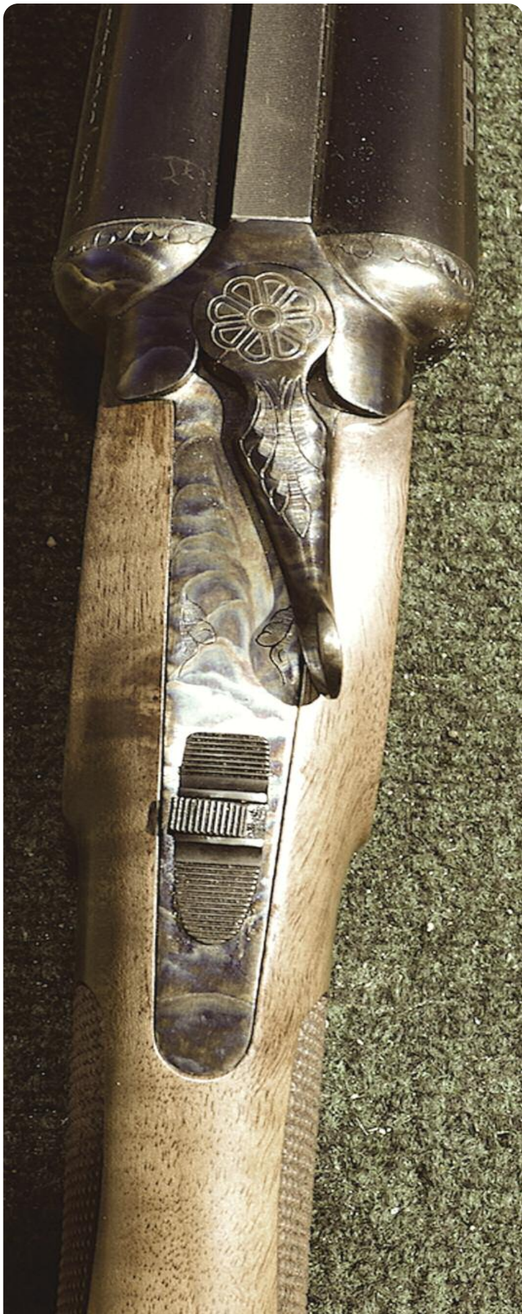
Lever angled slightly to the right. The manual safety houses the barrel selection switch.
