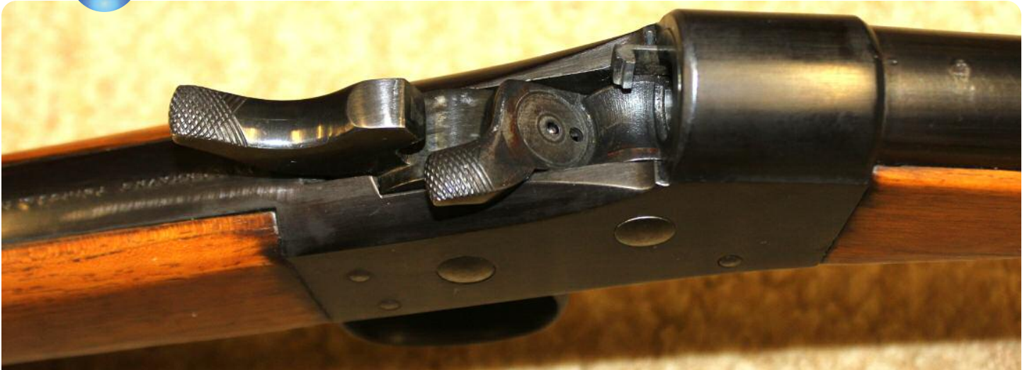
The breech of a Danish Rolling Block. Notice two holes in block for the rim fire firing pin and the center fire firing pin.
