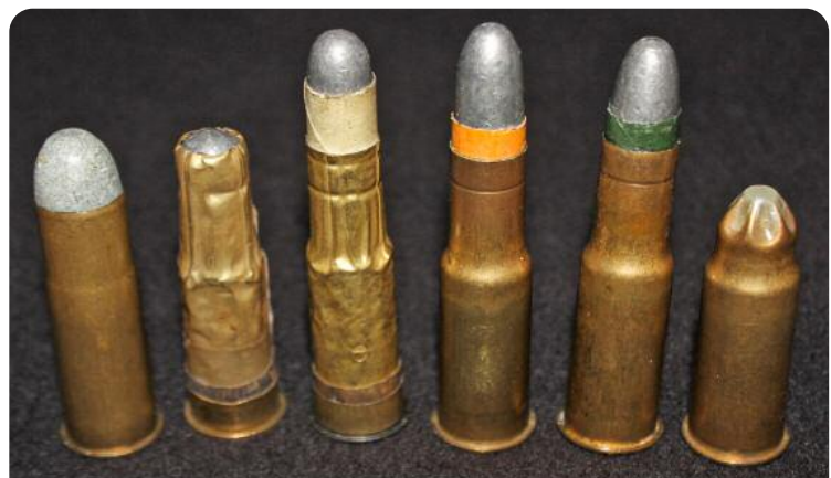
Left to Right—Snider .577 with 480-grain bullet, parent cartridge to the Martini-Henry cartridge; Coiled-Rolled Brass Foil M-H Buck Shot round; Coiled-Rolled Brass Foil Paper Patched 480-grain M-H round; Standard Paper Patched 480-grain Drawn Brass M-H round; Paper Patched 400-grain M-H round; M-H Blank round.
