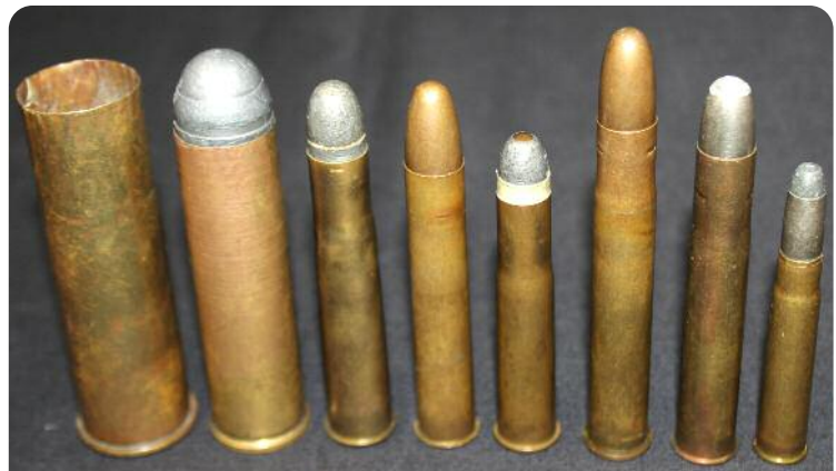
Sporting Cartridges Left to Right—4 bore case; 8 bore; 577/500 Nitro Express; 500 Nitro; 500/450 # 1 Express; 475 # 2 Nitro; 470 Nitro; 9x57mmR.
