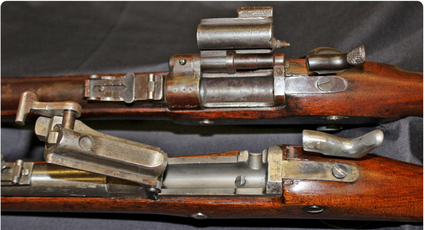
Top—The Snider-Enfield hinged breech. Bottom—The Springfield 1873 Trapdoor hinged breech.
