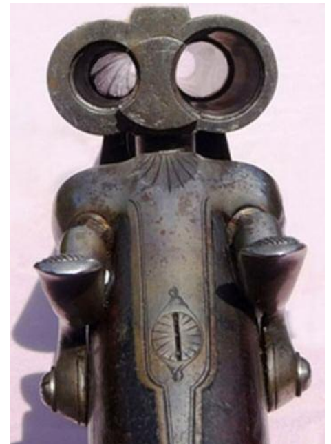
One style of combination gun, the Cape Gun, showing rifling in the left barrel and a smooth left barrel.
