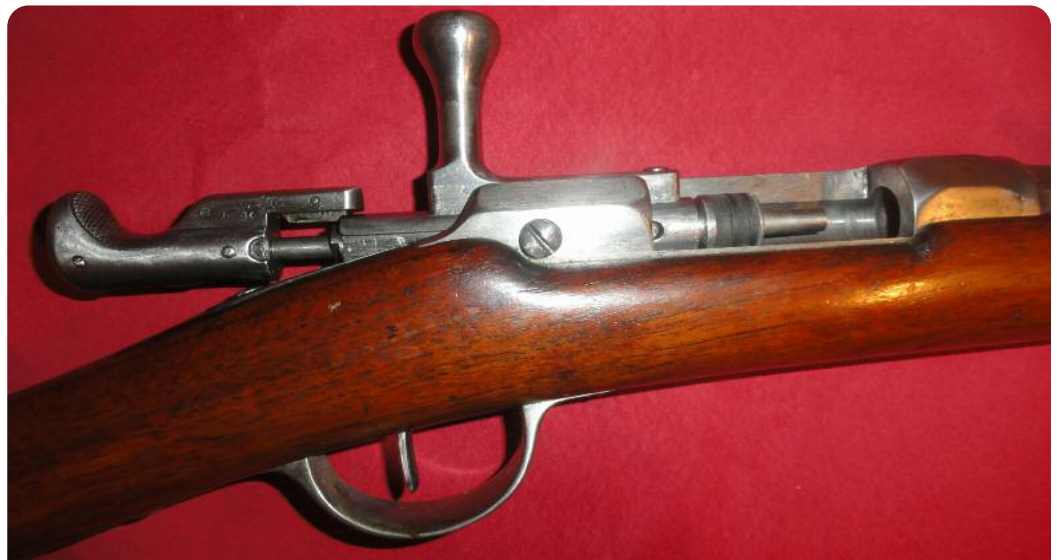
The French Chassepot Needle Rifle with bolt open showing part of firing pin assembly.
