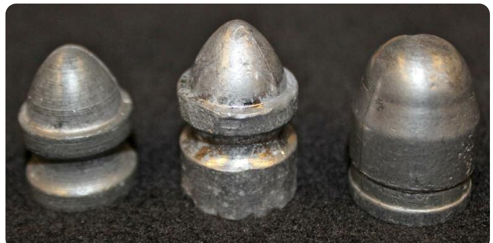
Solid bullets for an 8 gauge/bore—Left to Right 1,020-grain, 1,350-grain, 1,500-grain.
