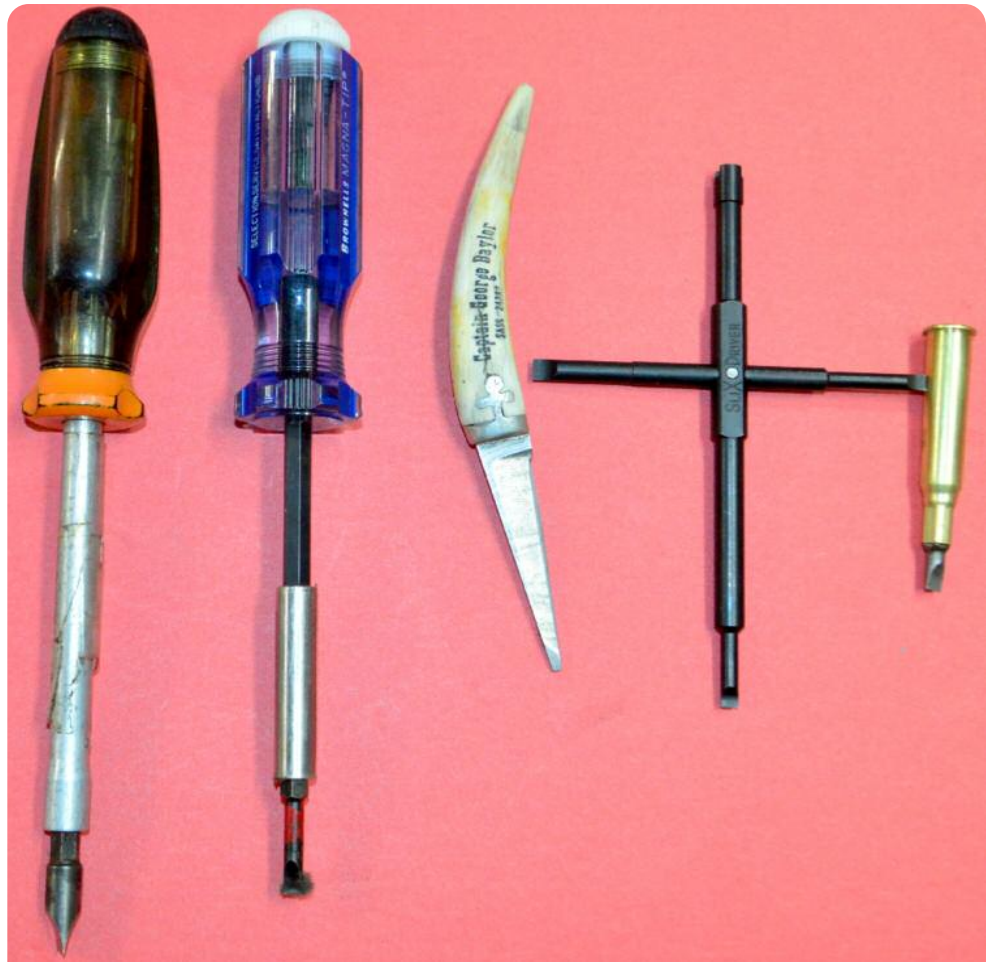
Screwdrivers from my gun cart, left to right: a Lyman handle with tips from a Magna-Tip thin bit set (Brownells 080-120-000WB) for Uberti '73; Ruger® Screwdriver Set (Brownells 080-000-020WB); Redwing Frontiersman Screwknife©; SliX-Driver with nipple wrench, Cowboy screwdriver for gun belt.
