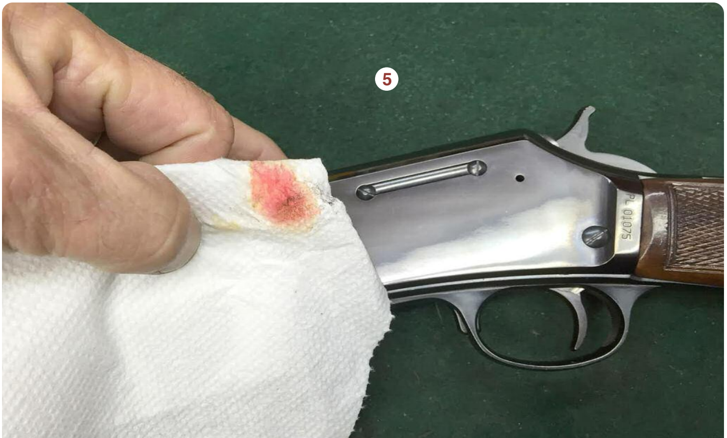
Fig. 5— Testing the side frame of this Lightning proved positive for the presence of lead after 60 rounds were fired. The area swabbed was 28" from the muzzle.
