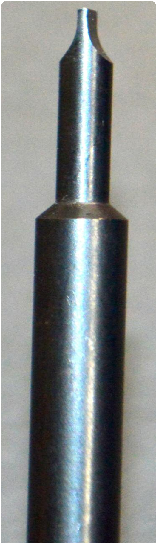
One of the hollow ground screwdriver tips on the SliX-Driver.
