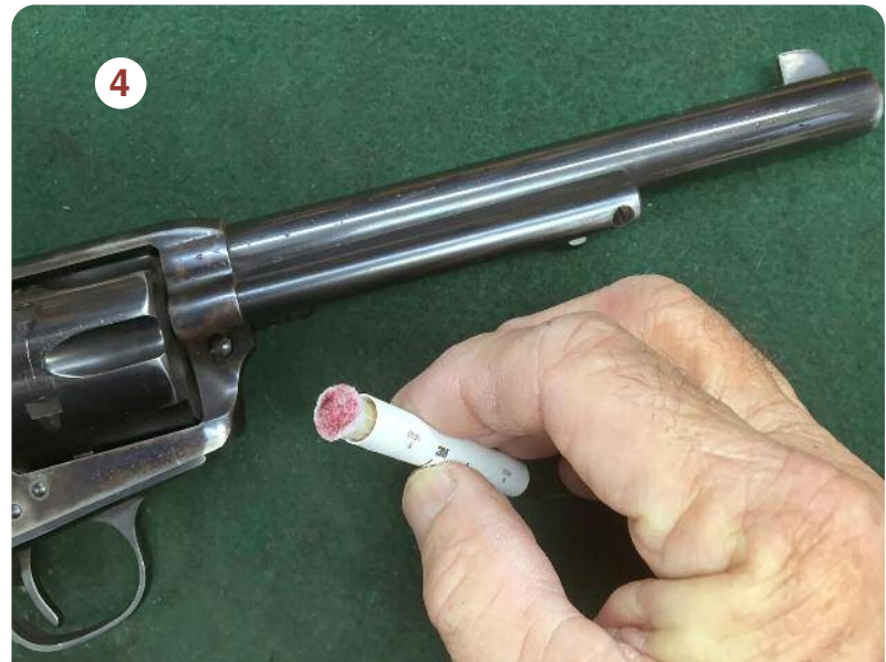
Fig. 4—The side of the barrel above the ejector on this SAA proved positive for the presence of lead after only 30 rounds were fired.
