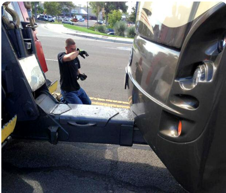
In 2015 the oil pump failed and took a lot of parts with it. No flatbed in Albuquerque, so a huge wrecker arrived and towed it rear wheels on the ground (drive shaft disconnected).
