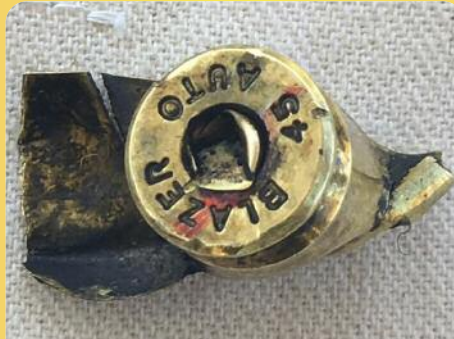
Close up of the primer shows indentation that matches the corner of the barrel hood.
