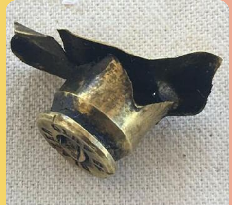
.45 ACP brass after out of battery discharge.
