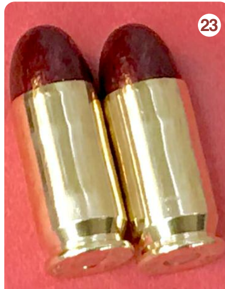
Typical .45 ACP cartridges that passed EGW checking., 230-grain RN polycoated bullets, light taper crimp, OAL case length 1.275" max.
