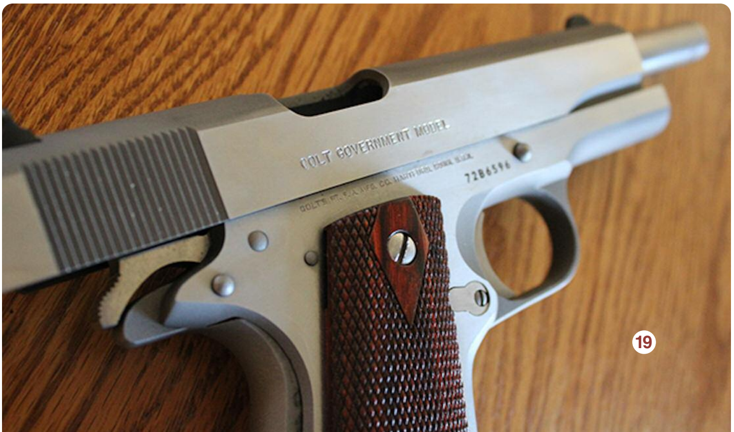
Standard “Mil-Spec” ejection port in Colt Series 70 1911A1. This will dent ejected brass. Lowering the ejection port is a legal cure for dented brass.
