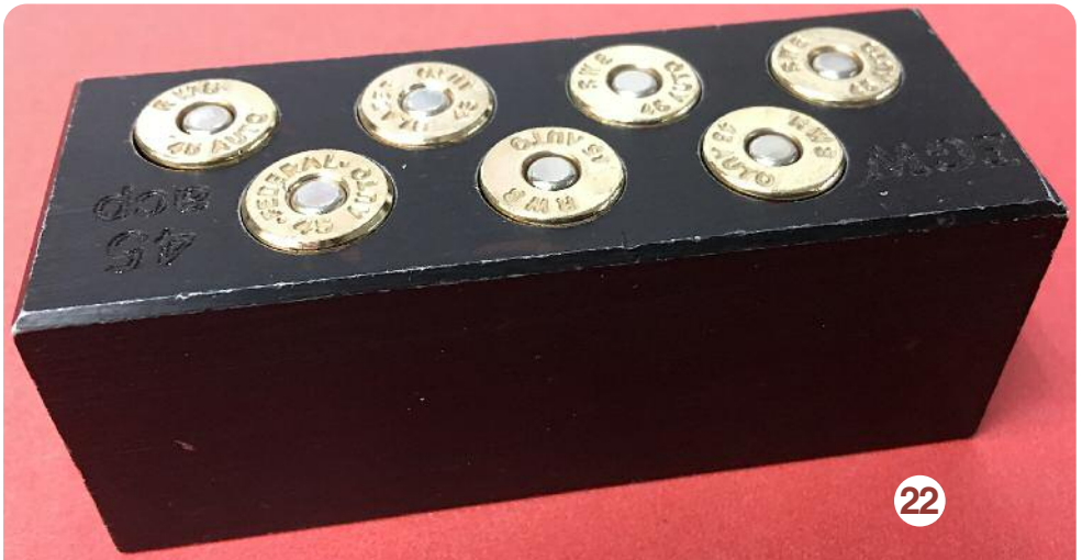
EGW case checker catches split cases, uncrimped rounds, bulged cases, and allows easy checking for high/upside down/missing primers.
