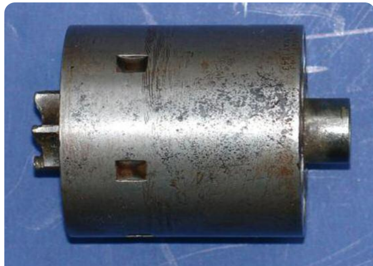
Flange on front of cylinder covers cylinder arbor to prevent fouling.
