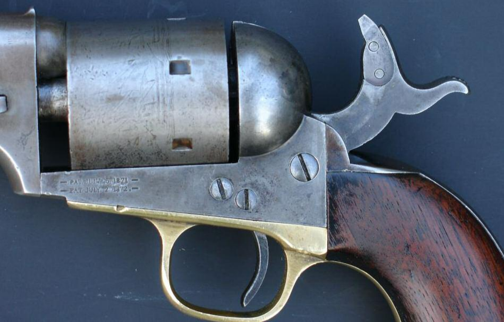
Side-mounted blade firing pin on 1872 Open Top.
