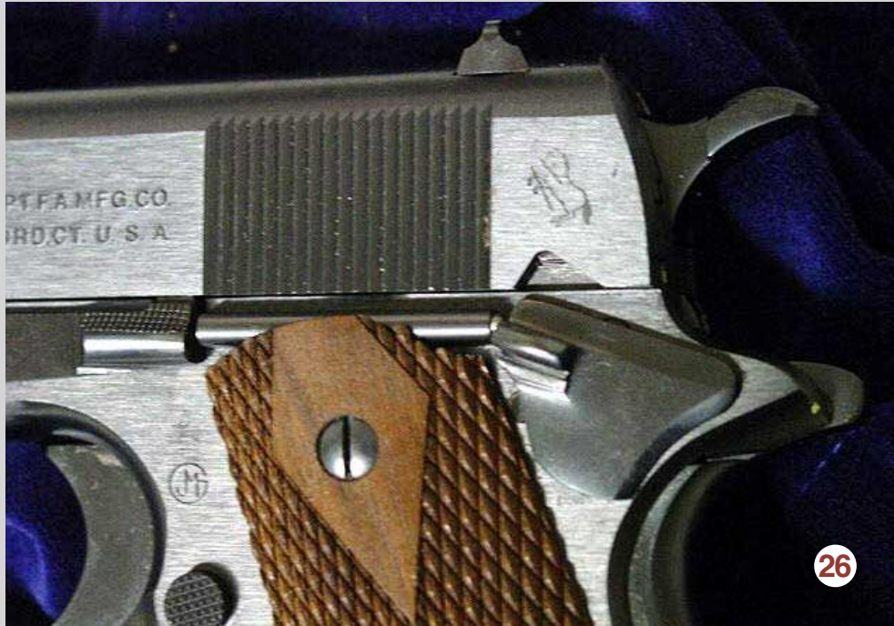
Original style grip panel on Colt 1911 WWI replica covers and protects the plunger tube.
