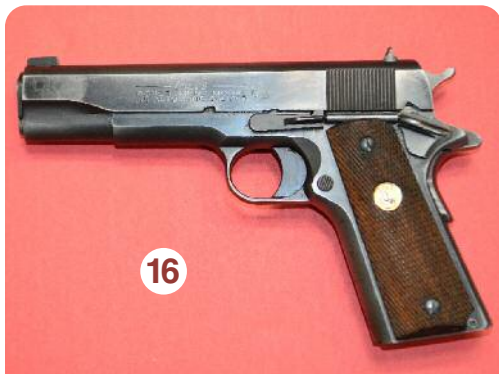
— Colt Series 80 1911A1 — a good Traditional Category gun out of the box. This one has visible modifications — dovetailed front sight and Wilson “Bullet Proof” Slide Release, checkered mainspring housing. Internal modifications include a crisp, light trigger, Wilson “Bullet Proof” extended ejector, Wilson “Bullet Proof” extractor, and firing pin.
