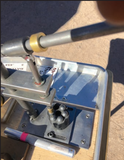
SEATING BALLS WITH CYLINDER LOADER.
