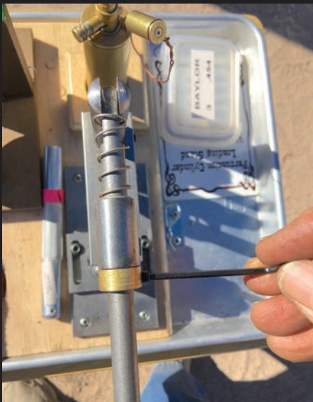
ADJUSTING THE BRASS COLLAR TO STOP AT THE LIGHTEST LOAD.
