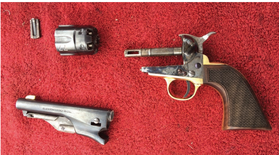
THIS IS AS FAR AS THE GUN NEEDS TO BE DISASSEMBLED FOR CLEANING BECAUSE THE INTERIOR OF THE FRAME IS FILLED WITH MOBIL 1 SYNTHETIC GREASE AND SEALED.
