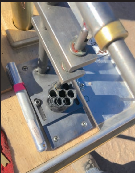
THE BALLS ARE SEATED TO THE LIGHT LOAD, WHICH THE RAMMER ON THE REVOLVER CAN'T DO.
