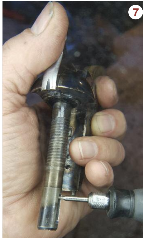
Breaking the edges of the wedge slot in the arbor.
