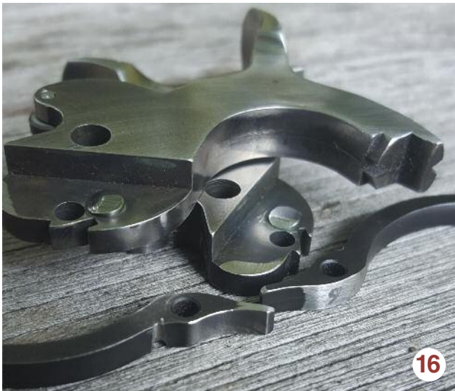
Cam height adjusted and polished. Trigger spring shelf removed and blended.
