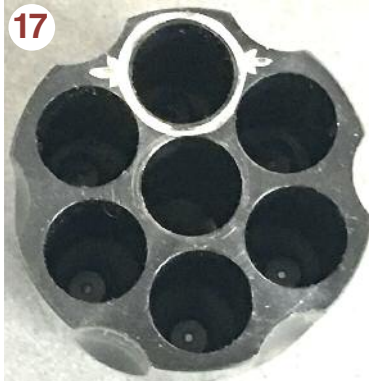
Aspen Filly engraved this empty chamber indicator and on the outside of the cylinder put the last 2 of the serial number to prevent misloading. Barrels got the last two numbers as well. When the numbers are lined up, the empty chamber is under the hammer.
