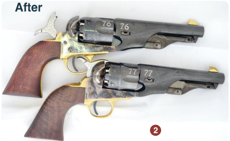
After Mike Brackett of Goon's Gunworks, did his extensive action work, Boomstick of Boomstick Arms Co., LLC. put Super Blackhawk hammer spurs on the hammers and Slick McClade of Slick Magic Guns, did the front sights, opened the notch of the rear sights, and jeweled the hammers.
