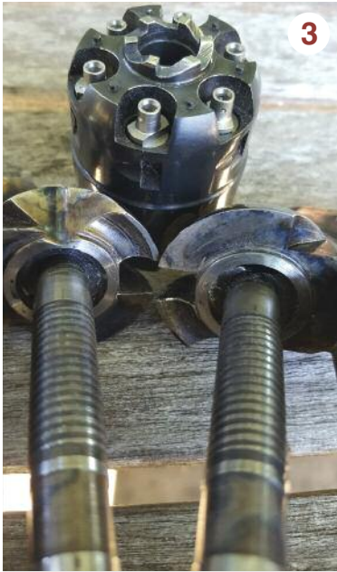
Recoil rings have been trued, arbors micro de-burred, cylinder ratchets cleaned up and polished. SliX-shot nipples replaced stock ones.
