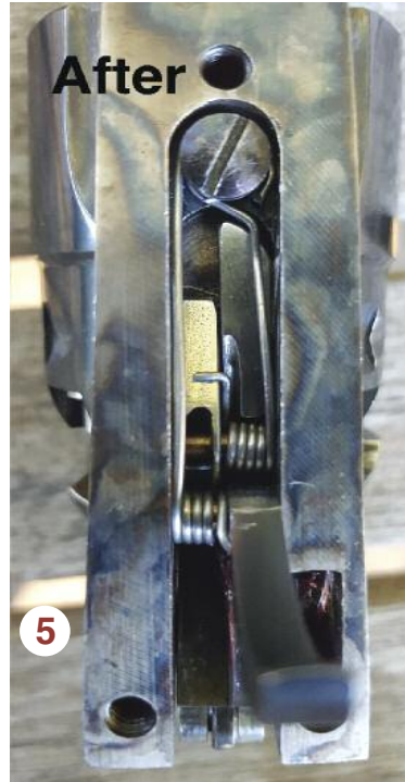
Torsion springs installed with bolt block in position.
