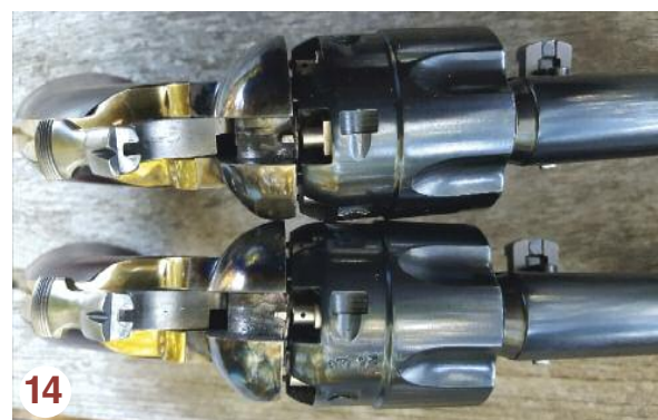
Top view showing cap posts installed and hammer faces de-burred and polished. Cap posts prevent spent caps from getting into the action.
