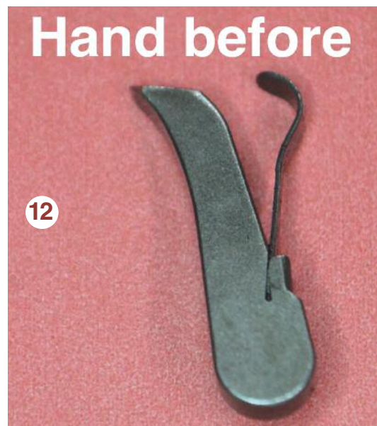
Stock hand with flat spring.
