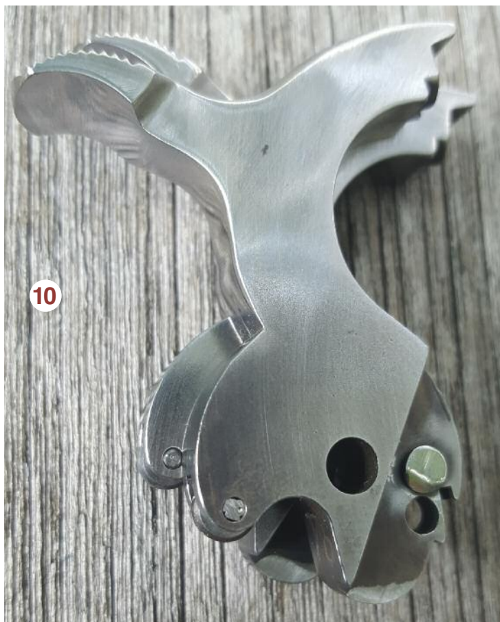
10 Hammer rollers "exposed" so they will contact the main spring roll slot fully.
