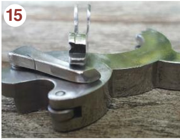
"This is some of the bolt detail. You can see the Munden step, which allows the bolt to enter the locking notch earlier than it normally would and my cutaway on the tall side. The top part of the cutaway has a back angle which protects the cylinder Locking notches." —Mike Brackett
