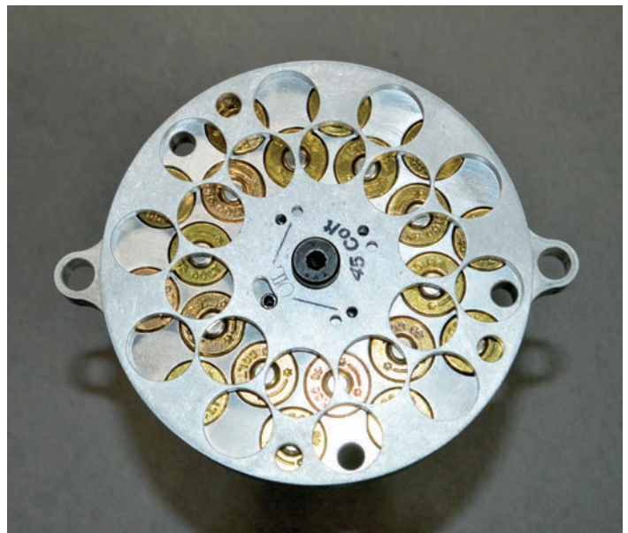
ST MACHINE LOADING BLOCK IN .45 COLT (ALSO AVAILABLE IN .38/.357). DROPPING A ROUND IN CATCHES UNCRIMPED ROUNDS, BULGED ROUNDS, SPLIT CASES, AND OUT OF SHAPE RIMS. AND... TURNING THE TOP PIECE CHECKS FOR HIGH PRIMERS.
