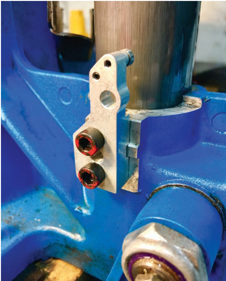
FOR BOTH THE DILLON SL900 AND THE XL650—A ROLLER BEARING REPLACEMENT FOR THE STOCK PART.
