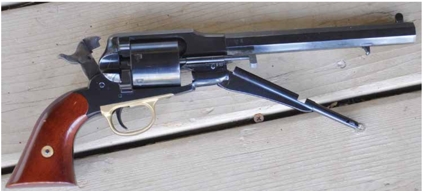
LOADING LEVER LOWERED TO ACTIVATE EJECTOR ROD.
