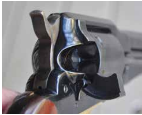
LOADING GATE AND CARTRIDGE CHANNEL OF CONVERSION.
