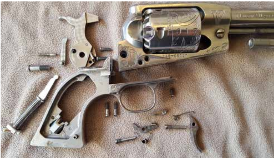
SOME OF THE WORK BY GOON'S GUNWORKS IS VISIBLE — LARGER PAWL SPRING AND PUSHROD, OPTIMIZED PAWL, MODIFIED BOLT, BOLT BLOCK, NEW TRIGGER SPRING, LIGHTER MAINSPRING, ADJUSTABLE ACTION STOP.
