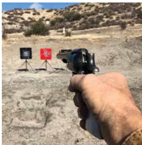
FIGURE 2. WHEN A RIGHT-EYE-DOMINANT PERSON CLOSES THEIR RIGHT EYE, THE IMAGE SEEN BY THE LEFT EYE REVEALS A QUESTIONABLY SIGHTED REVOLVER.
