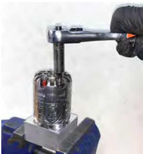
PHOTO 6 — CYLINDER BLOCK AND DEEP SOCKET NIPPLE WRENCH, BY KING SNAKE.
