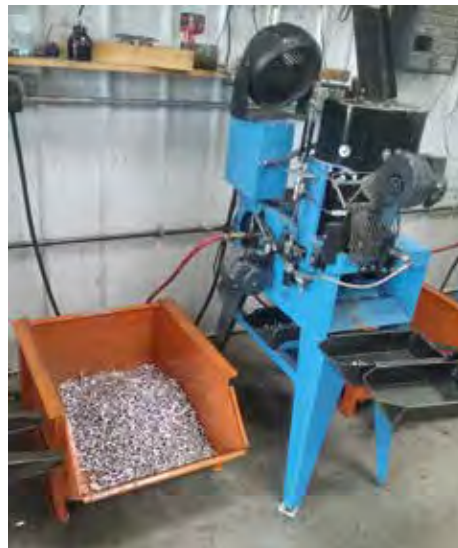
WHERE THE RUBBER MEETS THE ROAD. MOLTEN LEAD ON TOP IS SENT TO MOLDS, SETS, AND INTO THE TRAY FOR SIZING, LUBE, ETC.
