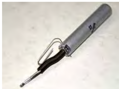
PHOTO 17 — ST MACHINING RUGER MAINSPRING COMPRESSOR WITH COMPRESSED RUGER OLD ARMY STRUT AND MAINSPRING. CUSTOM MADE CROSS-PIN NOT INCLUDED.
