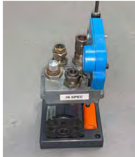
PHOTO 10 — PVC TOOL STAND FOR DILLON XL650 WITH PARTS NEEDED FOR CALIBER CONVERSION, BY KINGSNAKE.
