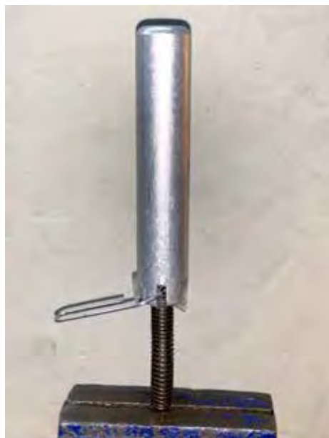
PHOTO 18 — ST MACHINING RUGER MAINSPRING COMPRESSOR MOUNTED IN A VISE FOR SPRING COMPRESSION. VISE NOT INCLUDED.
