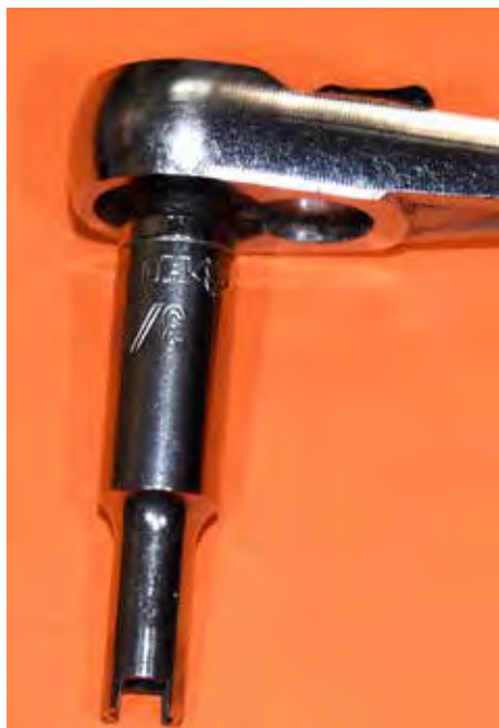
PHOTO 7 — 1/4" DRIVE 3/16" DEEP SOCKET CUT TO FIT REVOLVER NIPPLES, BY KING SNAKE.
