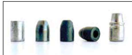
STEPS TO MAKING A BULLET (FROM THE LEFT): A CAST SLUG, A PRESSURE-FORMED BULLET MADE FROM THE SLUG (APPEARS DARK BECAUSE IT HAS BEEN TUMBLED), A COATED BULLET, A COATED HOLLOW-BASE BULLET, A MOLDED BULLET WITH A CANNELURE AND A TRUNCATED FLAT-NOSE TIP.
