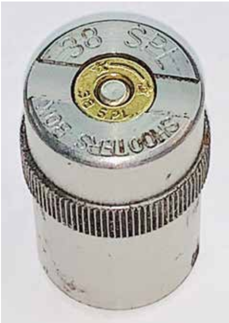
A ROUND IN A CASE GAUGE. IT WILL CATCH LACK OF OR POOR CRIMP, BULGES, BENT RIMS, AND SPLIT CASES.
