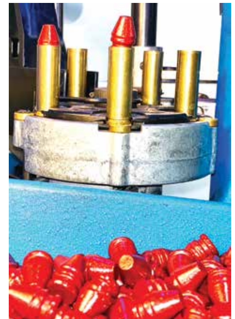
LOADING .38 SPECIAL 105-GRAIN COATED TRUNCATED CONE BULLETS ON THE DILLON XL650. STATION 1 - RESIZE CASE, DECAP; STATION 2 - PRIME, BELL CASE, INSERT POWDER; 3 - POWDER LEVEL CHECK; 4 - SEAT BULLET; 5 - CRIMP AND, WITH LEE FACTORY CRIMP DIE, RESIZE COMPLETED ROUND.
