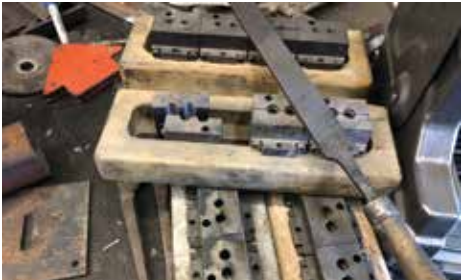
JUST A FEW OF THE MORE THAN 115 DIE SETS THAT STEVE USES TO CAST HIS BULLETS.
