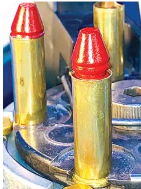
STATION 5 LEFT – BULLET INSERTED AND READY TO CRIMP; STATION 4 RIGHT – SLIGHTLY BELLED CASE WITH BULLET SITTING JUST INSIDE.
