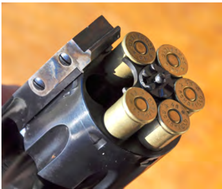
SCHOFIELDS EJECT ALL SHELLS AT ONCE, WHEN OPENED FULLY.
