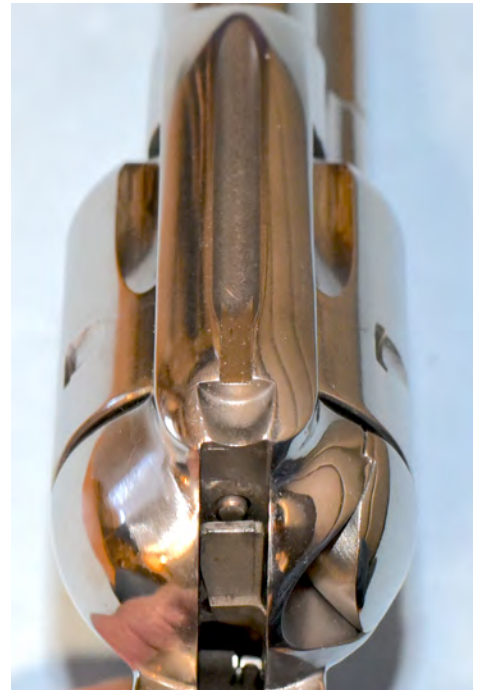
TRANSFER BAR IN THE "SAFETY" POSITION. HAMMER CANNOT STRIKE THE FIRING PIN.
