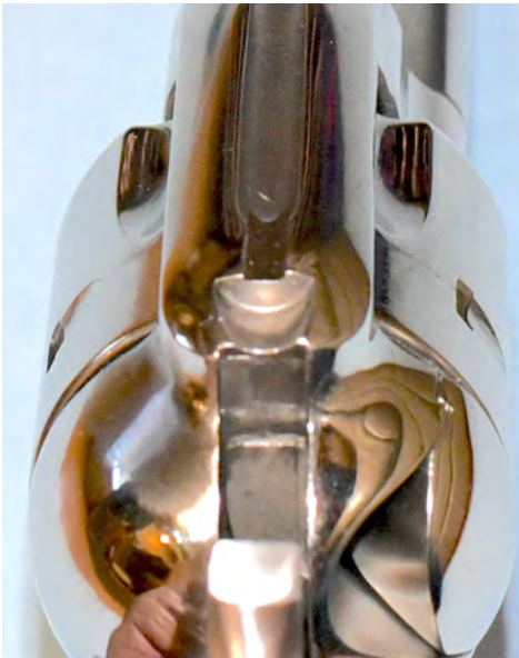
TRANSFER BAR LIFTS WHEN TRIGGER IS PULLED SO HAMMER FORCE IS TRANSFERRED TO THE TRANSFER BAR AND TO THE FIRING PIN, WHICH FIRES THE CARTRIDGE.
