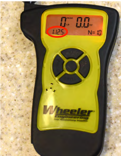
WHEELER ENGINEERING PROFESSIONAL TRIGGER PULL GAUGE SHOWING AVERAGE PULL OF 1 POUND 12.5 OUNCES FOR 10 PULLS. JIM CAN MAKE IT HEAVIER IF YOU WISH.
