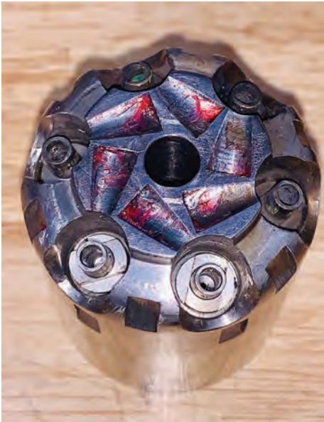
CYLINDER MODIFIED TO ALLOW LOADING WITH A CASH CAPPER AND WITH SLIXSHOT NIPPLES INSTALLED.
