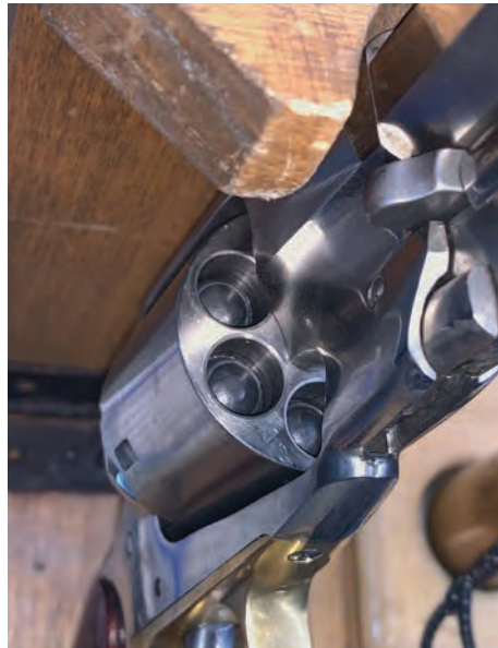
LOADED CYLINDER WITH 30 GRAINS OF GOEX 2F AND 147-GRAIN .457 ROUND BALL.
