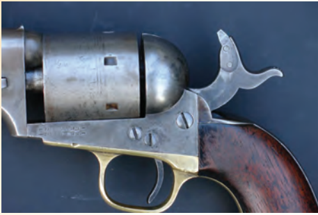
ORIGINAL 1872'S SIDE MOUNTED FLAT RIM FIRE FIRING PIN.
