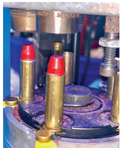
BULLET ON THE RIGHT IS SEATED. BULLET ON THE LEFT IS SEATED AND CRIMPED.
