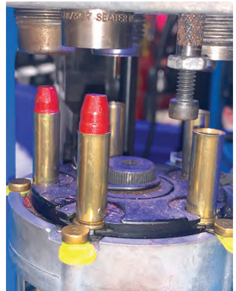
SET THE BULLET IN THE BELLING. USE ENOUGH BELLING TO AVOID SHAVING THE BULLETS AND NOT ANY MORE. KEEP THE BULLET IN PLACE UNTIL IT ENTERS THE SEATING DIE.
