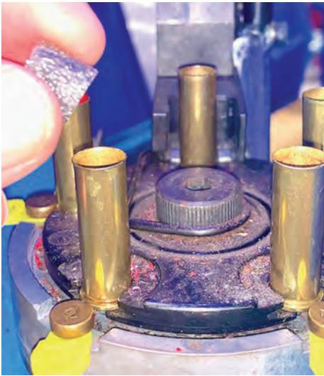
USING 3/8-INCH CAULK BACKER ROD FOR WADS/FILLER IN .38 SPECIAL TO FILL A SMALL AIR SPACE IN 11.8 GRAINS (WEIGHT) ONE CUBIC CENTIMETER AMERICAN PIONEER POWDER PREMIUM GRADE CHARGES. BULLETS ARE A NEW 105-GRAIN COATED TRUNCATED CONEFROM BULLETS BY SCARLETT. THEY ARE MEANT TO BE LOADED TO AN OVERALL LENGTH OF 1.484-INCH, PRIMARILY DESIGNED FOR '66 AND '73S FOR SMOOTHER CYCLING.
