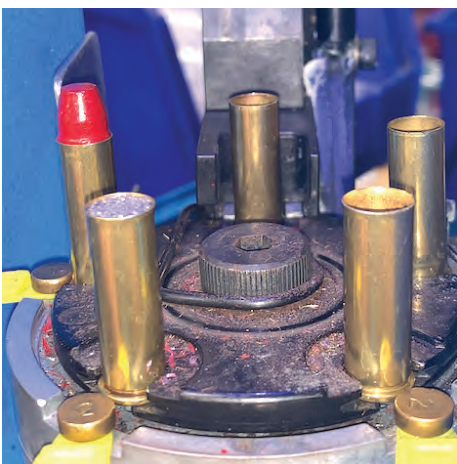
THE WAD MAY STICK OUT OF THE CASE. PUSH IN FLUSH. IF NEEDED, TURN A BULLET UPSIDE DOWN AND PUSH IT IN.
