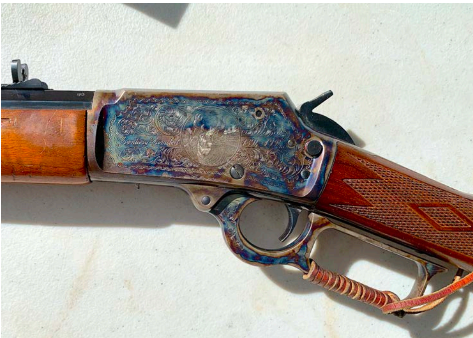
CENTURY LIMITED'S ENGRAVED RECEIVER WITH BONE COLOR CASE HARDENING BY DOUG TURNBULL (AUTHOR'S COLLECTION)
