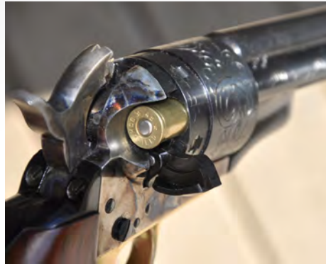
LOADING CHANNEL COMPLETED AND CONVERSION RING AND GATE INSTALLED.
