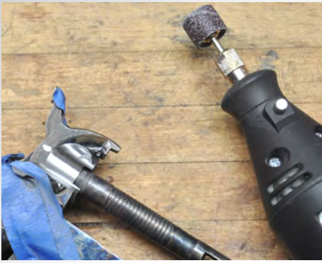
DREMEL DRUM USED TO CUT LOADING CHANNEL IN RECOIL SHIELD.
